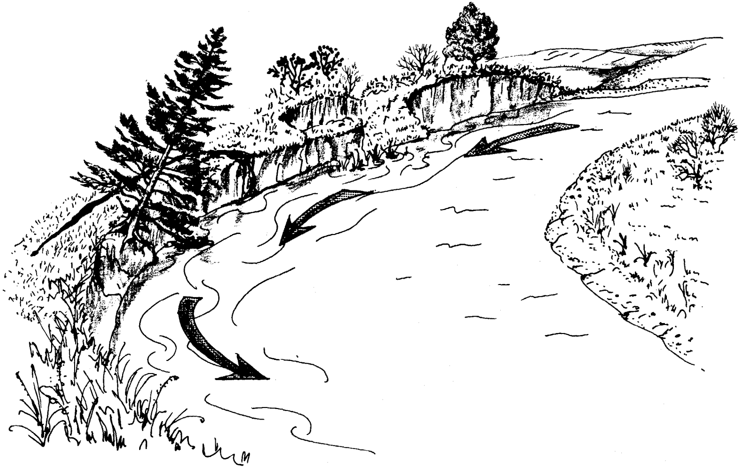
Figure 16. Active bank erosion exhibits fresh cut scarps, bankline cracks, slump blocks, and falling vegetation.
