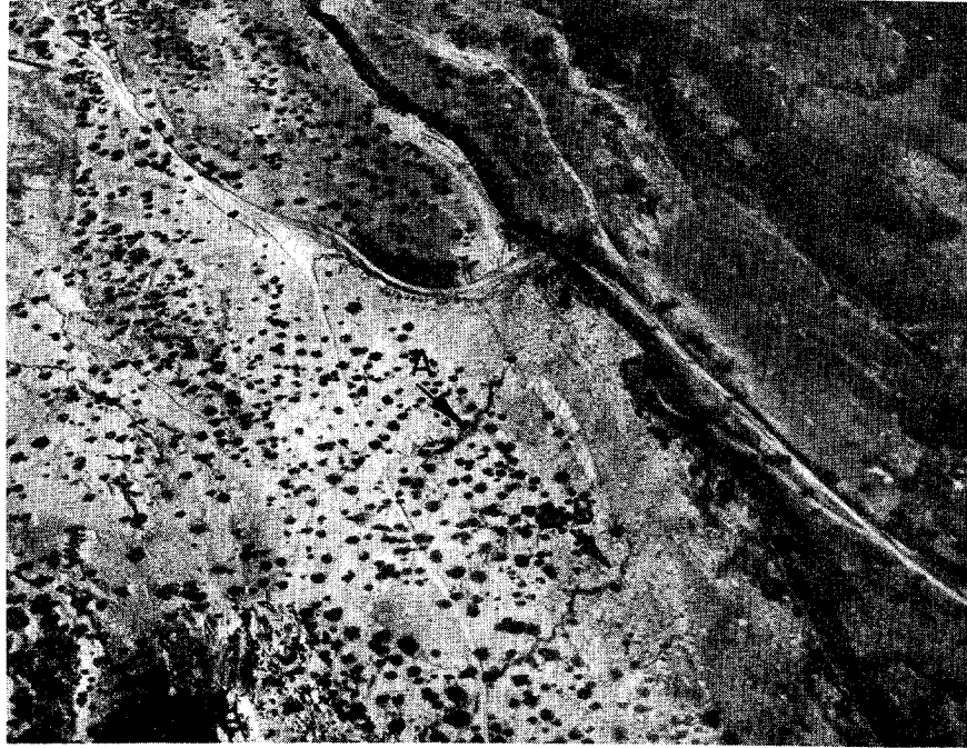
Figure 31. Evidence of Piping From Apparent Disappearance of Surface Drainage Features (Photo Compliments of Jay Lazarus, New Mexico Environmental Improvement Division).
