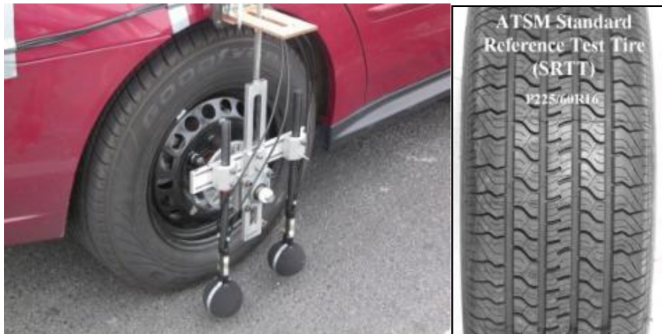
Figure 14. OBSI dual probe system and the SRTT.
