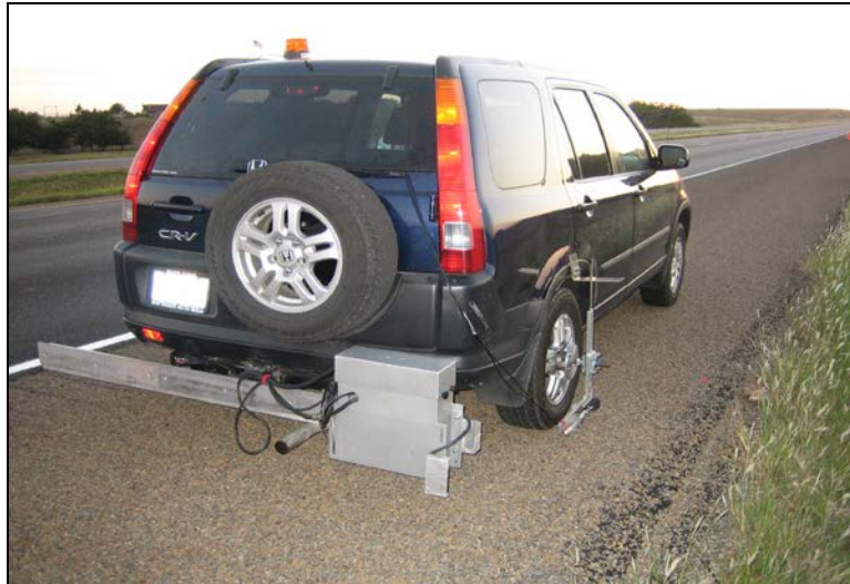
Figure 30. Laser profiler mounted behind the test vehicle.
