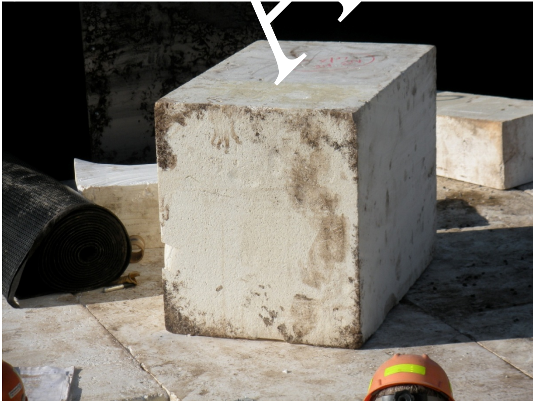
Figure 19. Photo. Close-up of EPS block.
