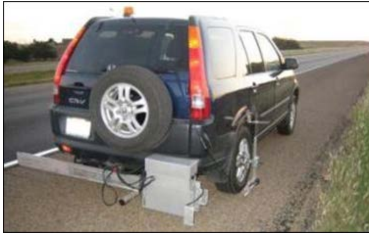
Figure 55. Photo. High-speed inertial profiler mounted behind the test vehicle.
