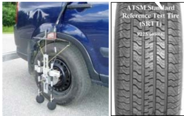
Figure 50. Photos. OBSI dual probe system and the SRTT.
