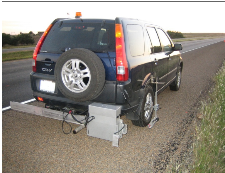
Figure 13. High-speed inertial profiler mounted behind the test vehicle.
