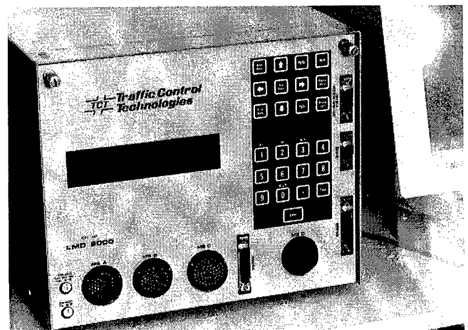
Figure II-8. TCT Model LMD 8000 Controller Unit
