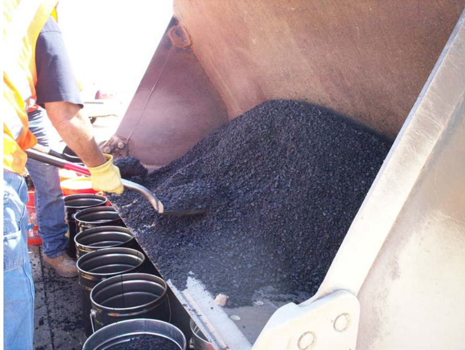
Figure 10. Photo. High-production sampling. (courtesy: Wyoming DOT)
