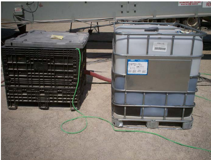
Figure 16. Photo. Additive system, Evotherm 3G added at 0.43 percent of binder. (courtesy: Wyoming DOT)
