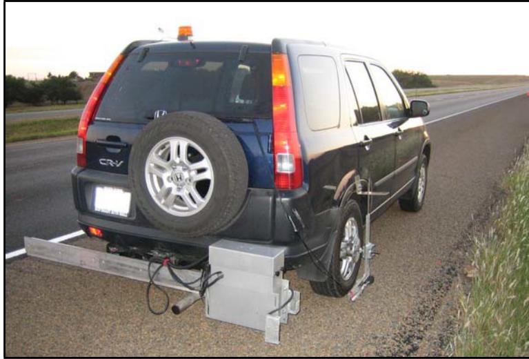
Figure 16. Laser profiler mounted behind the test vehicle.
