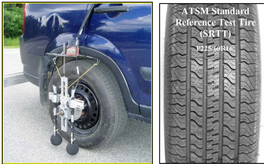
Figure 13. OBSI dual probe system and the SRTT.
