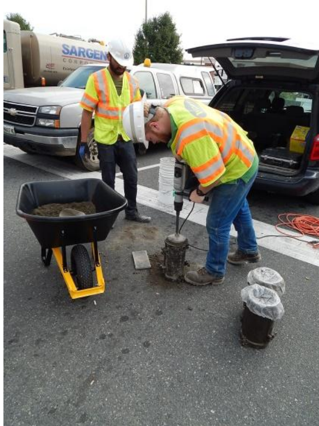
Top - Density testing using a nuclear gage, Bottom - Molding strength specimen Figure 12. Photos. Field testing during RCC placement.
