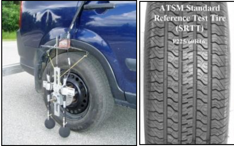
Figure 68. OBSI dual probe system and the SRTT.
