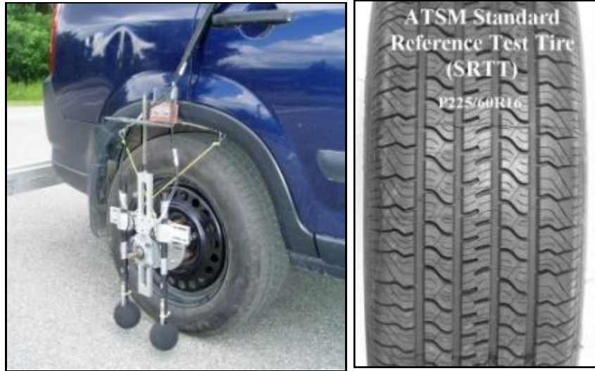
Figure 9. Photo. OBSI dual probe system and the SRTT.
