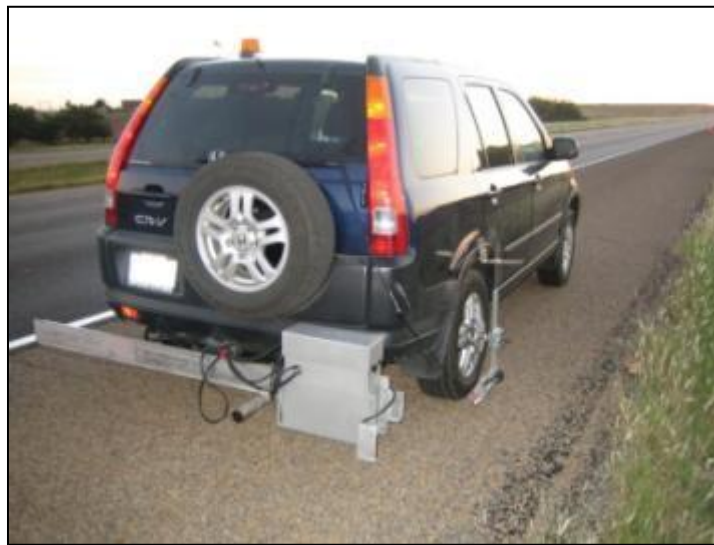
Figure 11. Photo. High-speed inertial profiler mounted behind the test vehicle.
