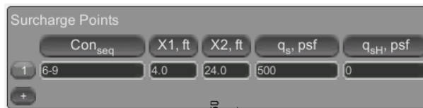
Figure 50. Screen Shot. Surcharge location and magnitude
