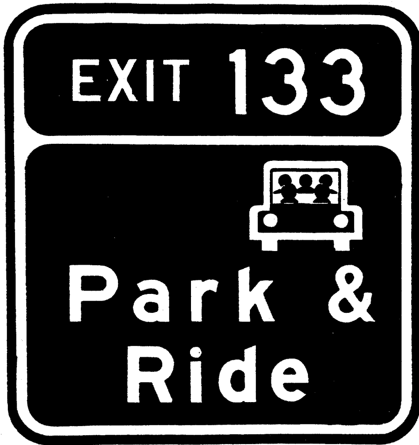
Figure 2E-20. Supplemental Guide sign for a park and ride facility (route with exit numbering).
