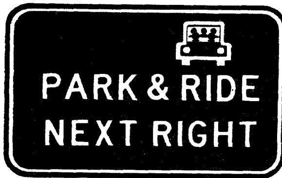
Figure 2E-19. Supplemental Guide sign for a park and ride facility (route without exit numbering).
