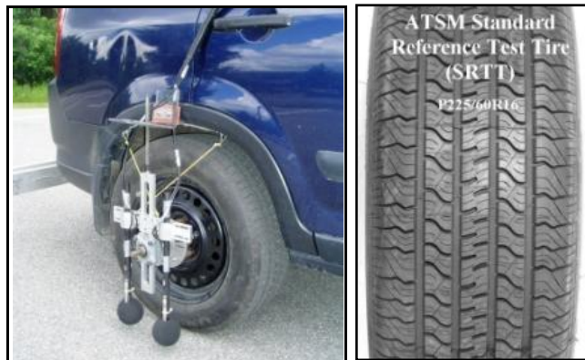
Figure 14. Photos. OBSI dual probe system and the SRTT.
