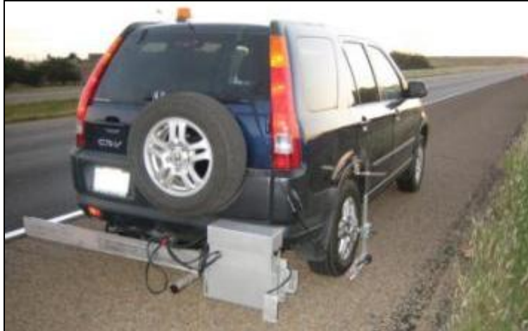
Figure 16. Photo. High-speed inertial profiler mounted behind the test vehicle.
