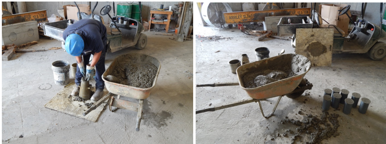
Figure 24. Photo. Testing of fresh concrete in the casting bay.
