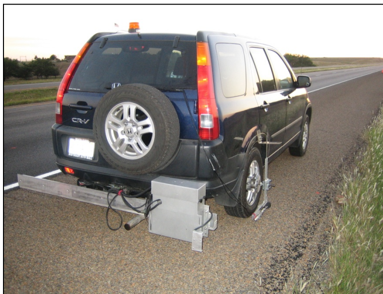
Figure 19. High-speed inertial profiler mounted behind the test vehicle.
