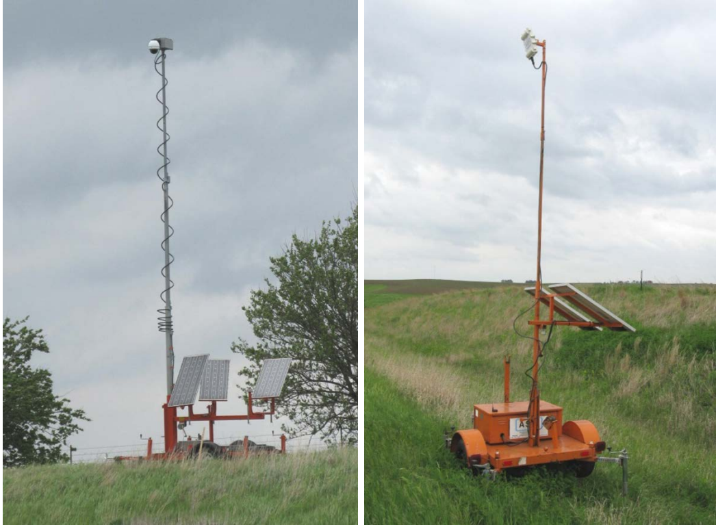
Figure 14. ITS portable camera (left) and the ITS portable sensor (right).
