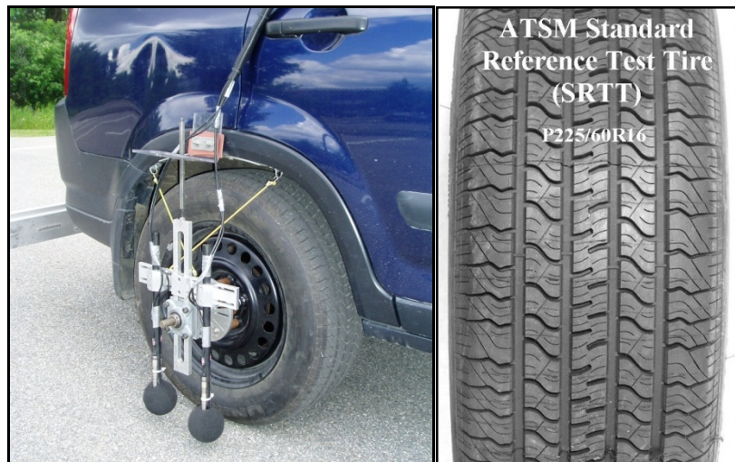
Figure 9. Photos. OBSI dual-probe system and the SRTT.
