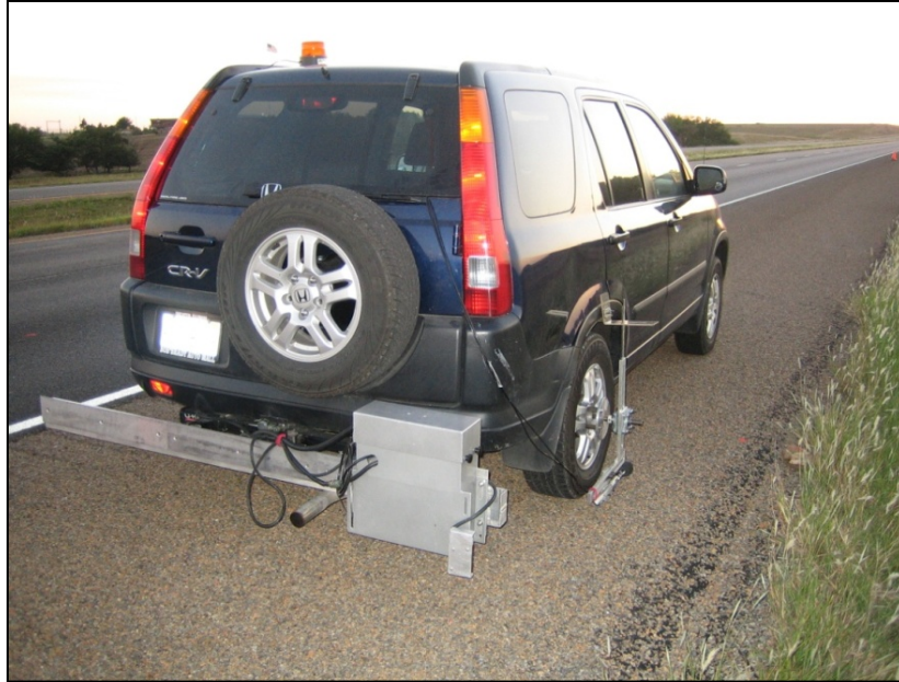
Figure 8. Photo. High-speed inertial profiler mounted behind the test vehicle.
