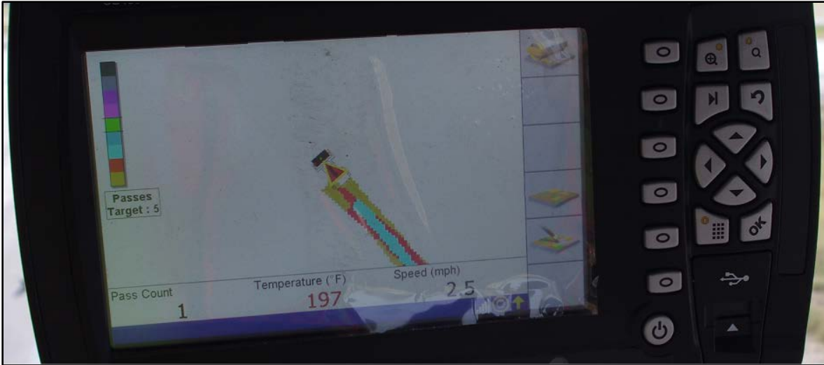
Figure 6. Photo. Onboard computer screen showing color-coded display of roller passes.
