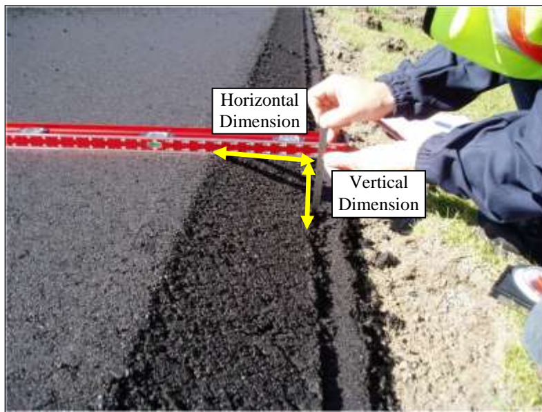
Figure 2. Slope measurement technique.
