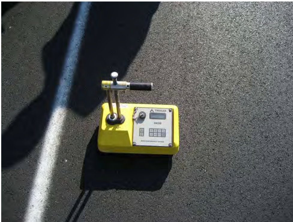
Figure 8. Troxler 3430 nuclear density gauge used to measure WMA density.
