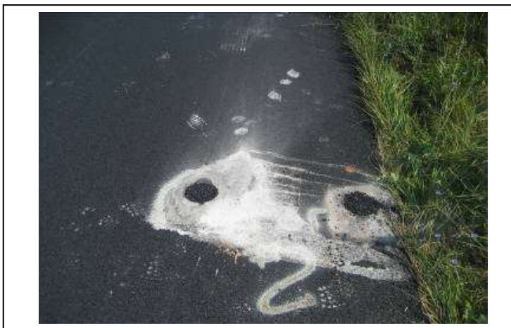
Figure 10. Location of cores and nuclear density tests.
