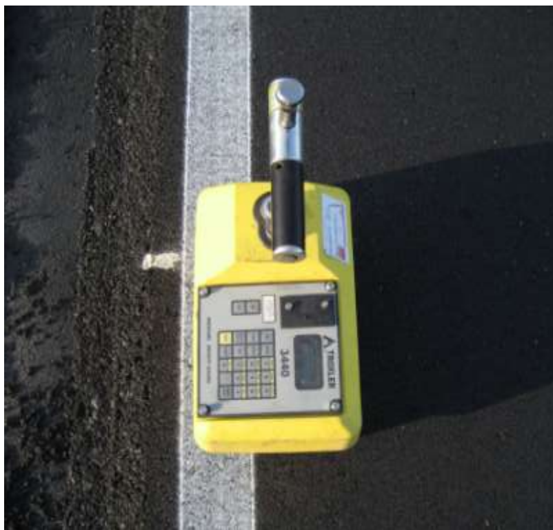
Figure 7. Troxler nuclear density gauge used to measure HMA density.
