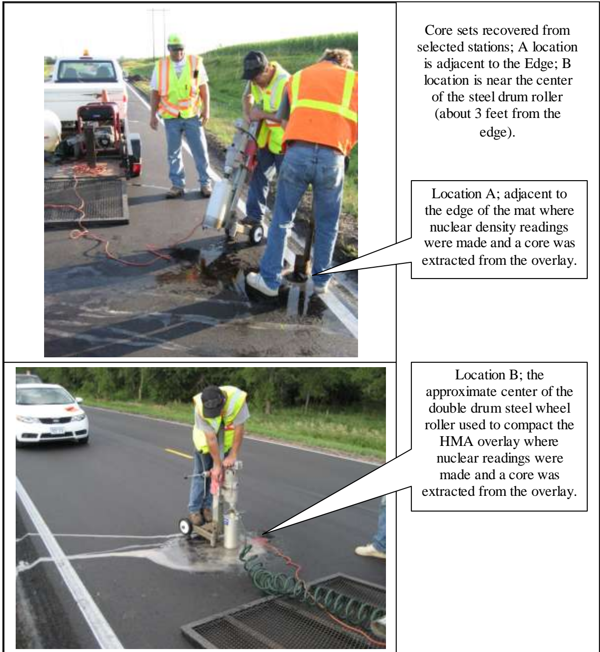
Figure 9. Photos show location of cores and nuclear density tests made with the Troxler gauge (nuclear density readings were taken and then the overlay was cored).
