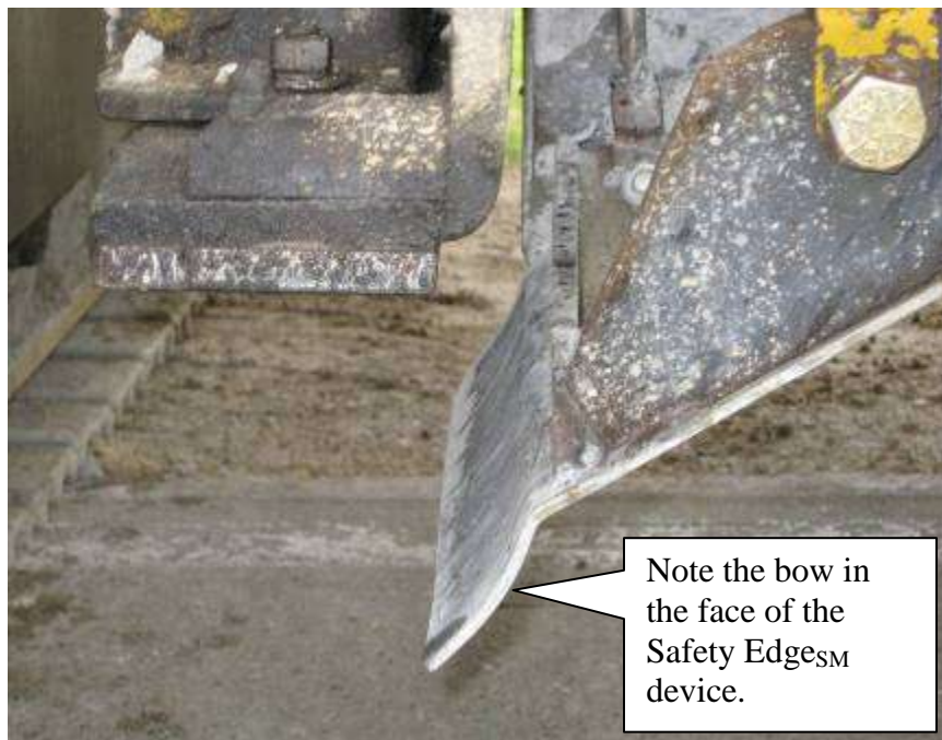
Figure 15. Viewed from the rear of paver showing the bend in the Safety Edge SM device.
