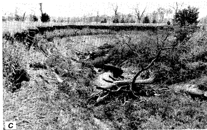
Figure 147. Middle Creek at site 70. A, Airphoto of site in 1955, position of relocated channel shown in dashed line. (From U.S. Dept. of Agriculture) B, View upstream along relocated channel from beneath bridge, in 1979. Top of exposed pier footing is at left. C, Bank erosion at bend upstream from relocated channel, in 1979. Bank height is 7.5 m.
