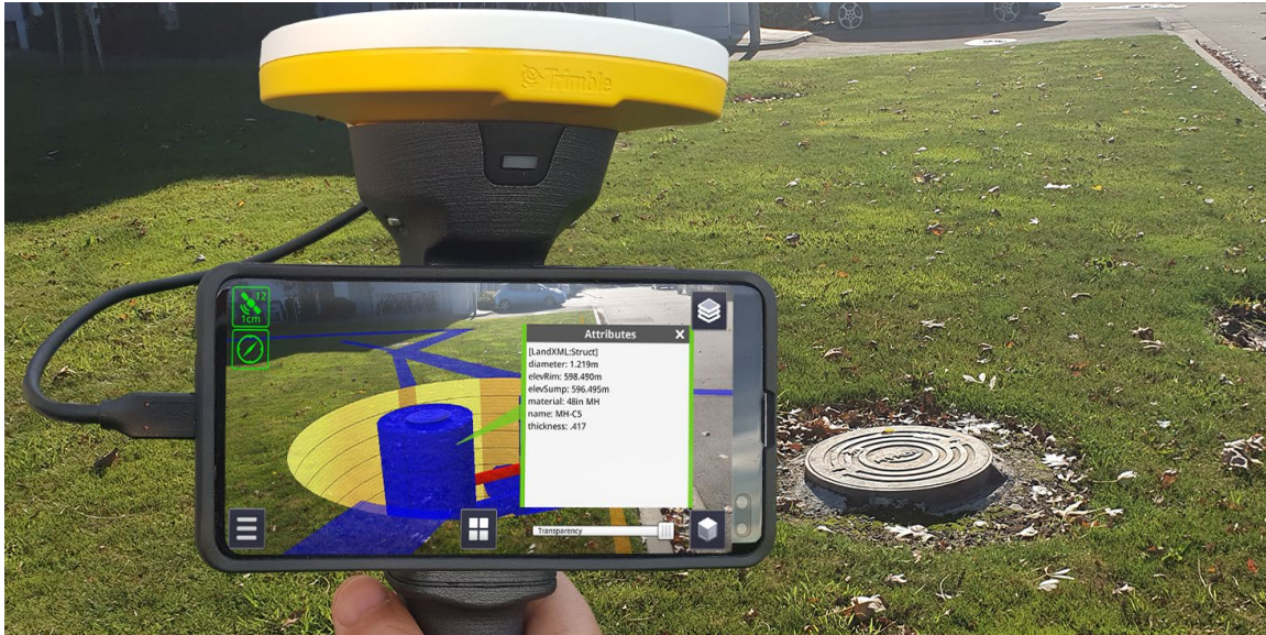
Figure 9. Photo. Display of 3D MEP overlaid on the video display of a tablet device.
