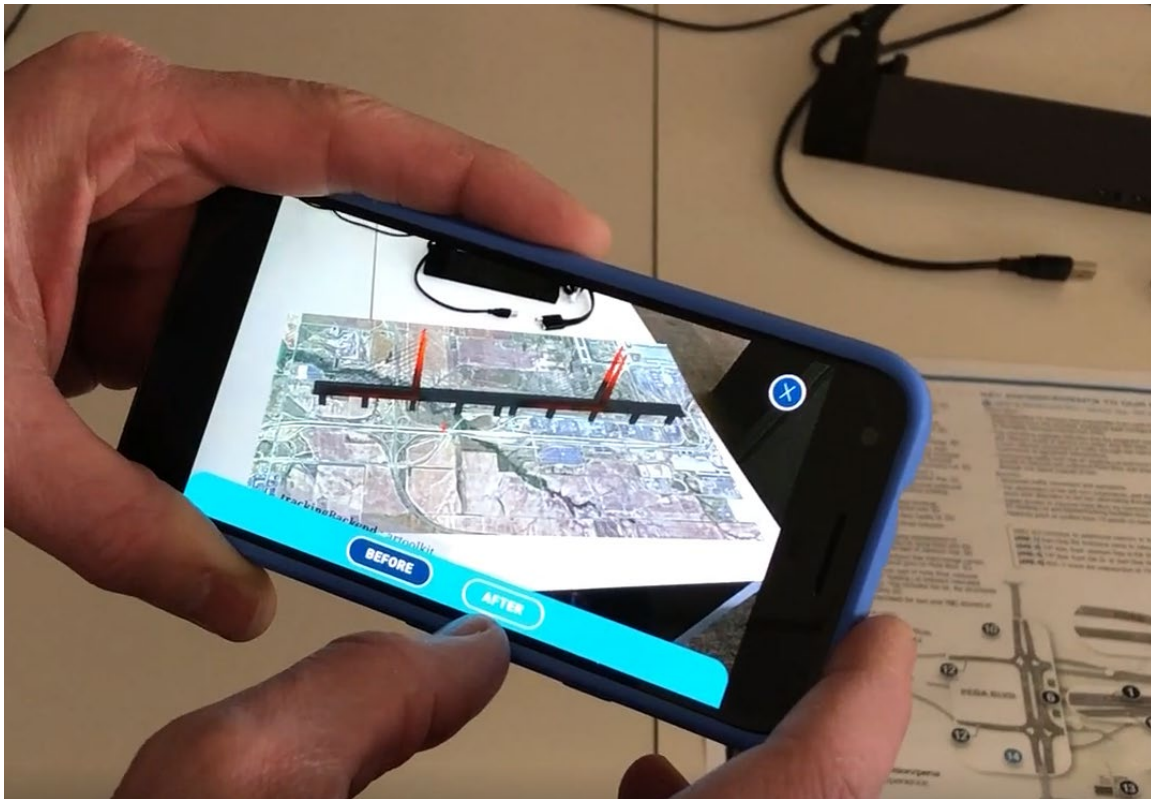
Figure 6. Photo. 3D view overlaid on live video on a mobile device.
