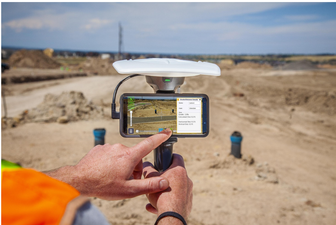
Figure 4. Photo. Handheld AR tablet device with GNSS tracking hardware.
