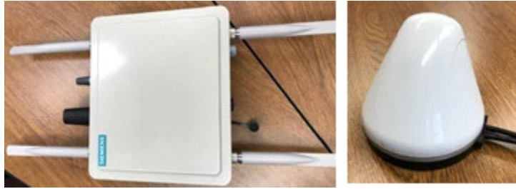
Figure 3.3. RSU (left) and OBU (right)
