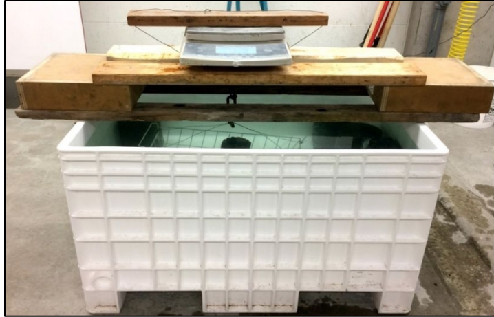
Figure 3.3. Water bath for submerging specimens for porosity testing
