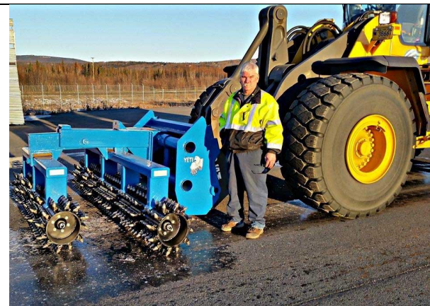
Figure 6. The Yeti icebreaker custom built for use at Fairbank International Airport. Source: http://dot.alaska.gov/comm/pressbox/arch_2015/PR15-2554.shtml# ( https://www.youtube.com/watch?v=XJiWOByFMil )
