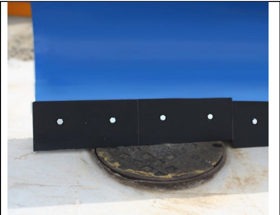
Figure 20. Multi-Segment Cutting Edge Source: https://www.kageinnovation.com/
