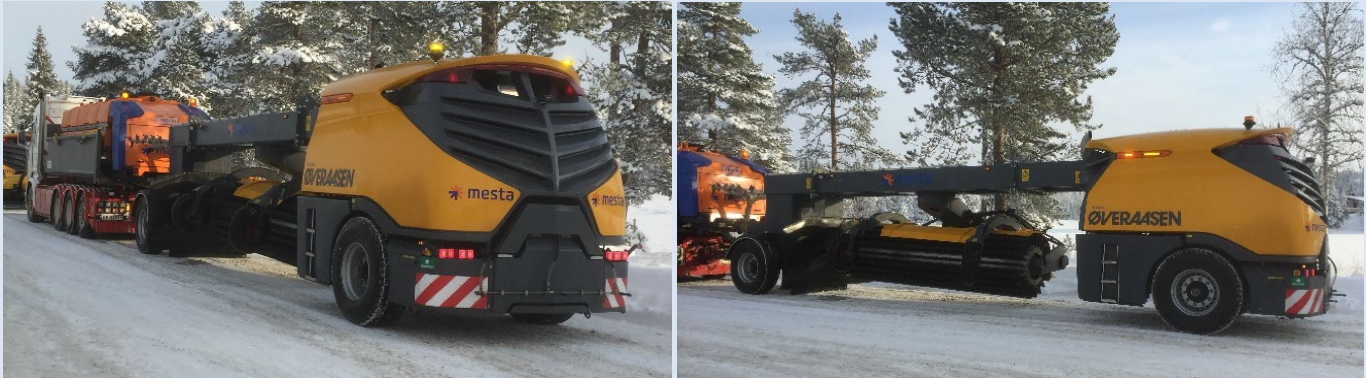
Figure 23. Another example of a tow behind sweeper used in Norway. Source: Norwegian Public Roads Administration
