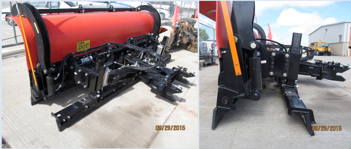
Figure 12. SDDOT squeegee blade set-up. Source: SDDOT, D. Varilek.
