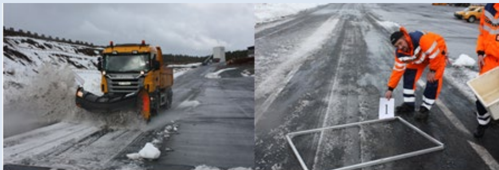
Figure 19. Field test, plowing slush with rubber blades at 40 mph; left before, right after showing data collection. Photos provided NPRA.
