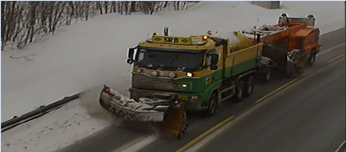
Figure 22. Norwegian snow plow with tow behind sweeper. Source: Norwegian Public Roads Administration
