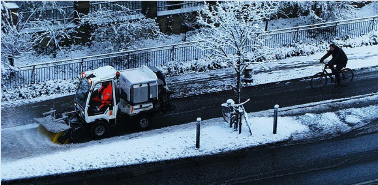
Figure 24. The use of smaller scale sweepers to manage snow on pedestrian and cycle paths in Norway. Source: Norwegian Public Roads Administration
