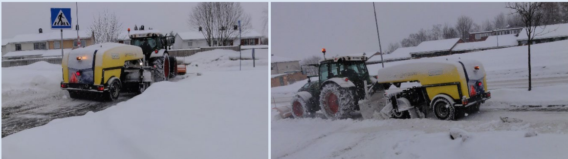
Figure 25. A tow behind sweeper attached to a tractor, used to clear snow for pedestrian traffic on sidewalks. Source: Norwegian Public Roads Administration
