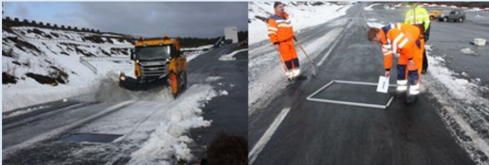
Figure 18. Field test, plowing slush with rubber blades at 25 mph; left before, right after showing data collection. Photos provided by NPRA.
