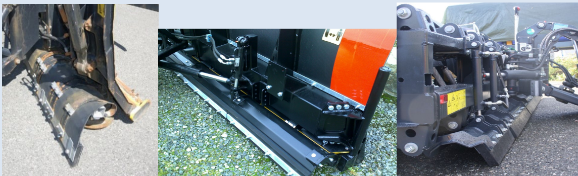
Figure 16. From left to right, NPRA slush blade, Arctic Machine slush blade, Schmidt segmented slush blade.
