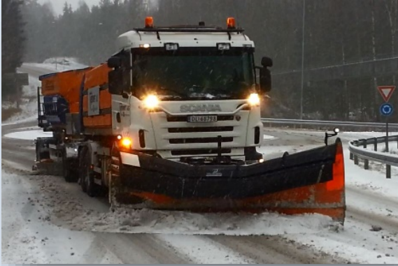
Figure 13. Snowplow vehicles with tow behind trailers with slush blades used by the Norwegian Public Road Administration. Source: Tellefsdal/AEBI/SCHMIDT
