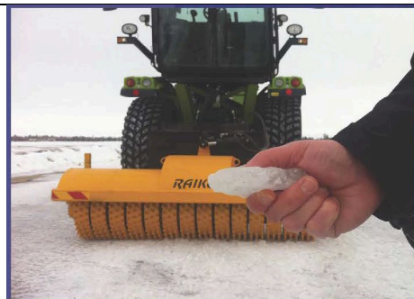
Figure 7. Raiko T model IceBreaker. Source: http://team-eagle.ca/equipment/raiko/
