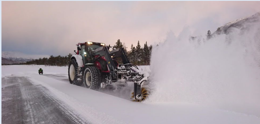
Figure 26. Field research investigating the travel speed and the use of front mounted sweepers for winter maintenance operations in Norway. Source: Norwegian Public Roads Administration
