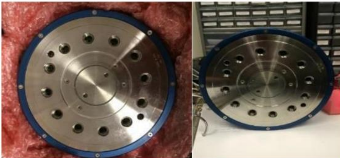
Figure 11: Pictures of 6 degrees of freedom loadcell
