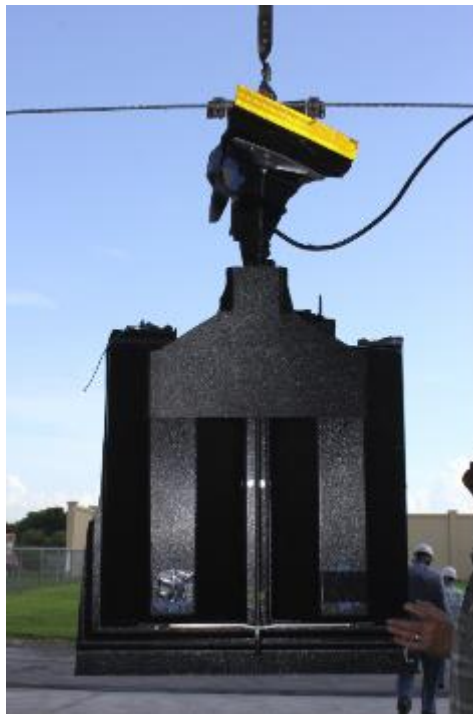
Figure 57: 5-section signal after completion of test
