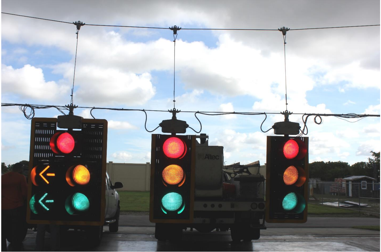
Figure 75: Signal assemblies installed on test frame (before testing)
