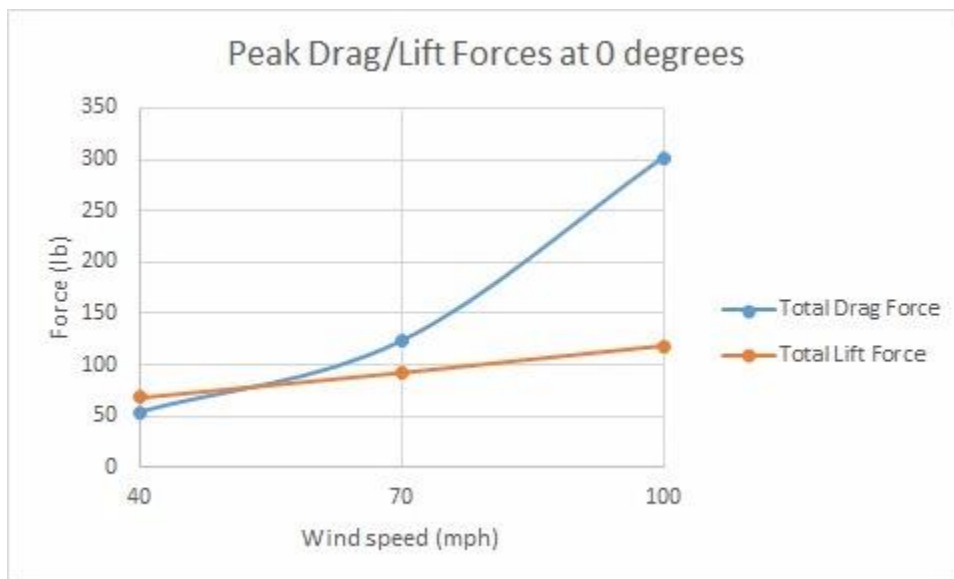
Figure 160: Drag ( F_y ) and lift ( F_x ) forces on the traffic signal at 0 degrees: a) Mean; b) Peak
