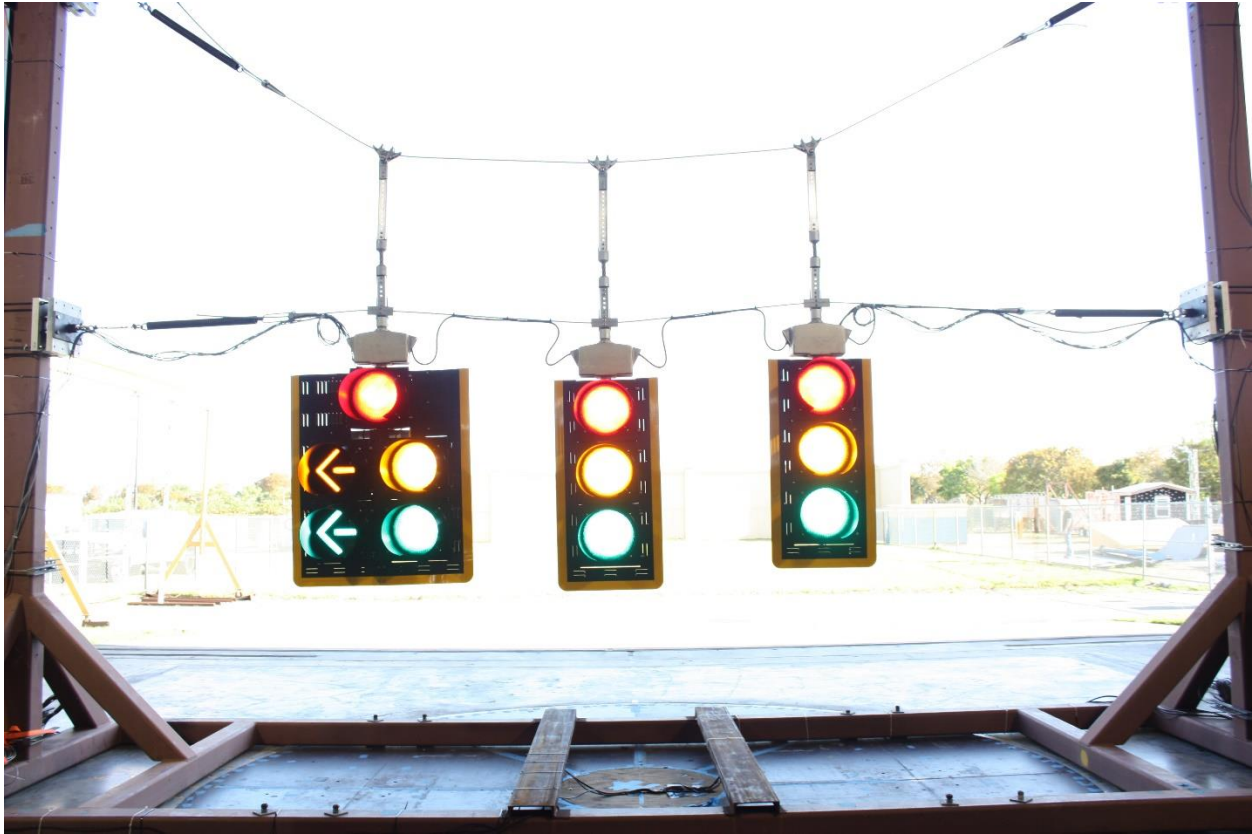
Figure 118: Signal assemblies installed on test rig (before testing)
