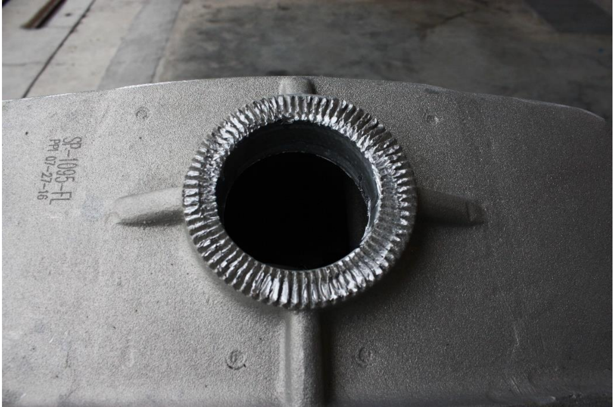
Figure 132: 5-Section signal disconnect box with damaged serrated teeth
