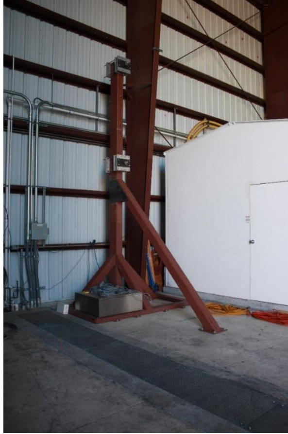
Figure 4: Reinforced long span test rig
