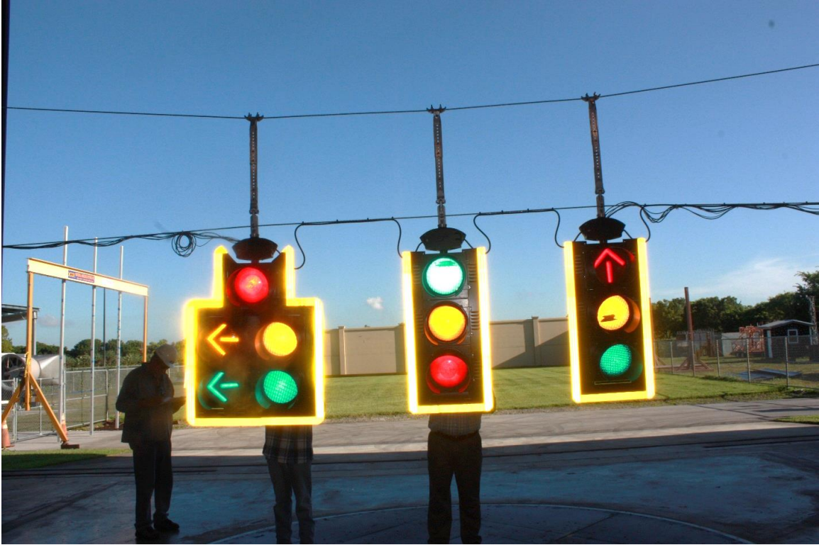
Figure 103: Signal assemblies installed on test rig (before testing)
