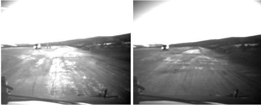
Figure 1.4 The captured test samples. Left-hand image is captured with a horizontal polarization filter and the right-side image with a vertically polarized component. (from Kutila et al. 2008)
