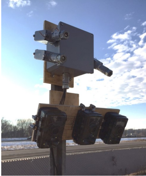
Figure 2.3 Monitoring setup at the permeable asphalt test section: gray box at top is the enclosure and mount for the 3 infrared sensors; 3 trail cameras (two with polarized lenses) are mounted below the enclosure.
