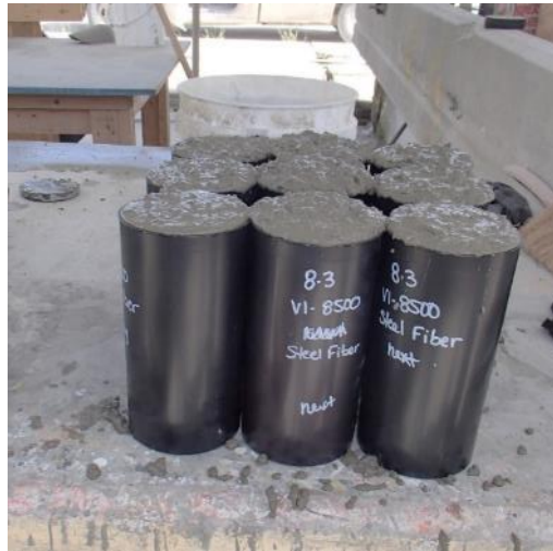
Figure C-3 Cylinders for testing of compressive strength
