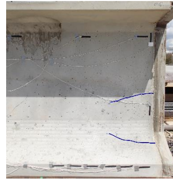
Figure 5-43 End region cracking after prestress transfer for PP-50 specimen: (a) analytical and (b) experimental.
