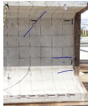
Figure 5-42 End region cracking after prestress transfer for CR-70 specimen: (a) analytical and (b) experimental.
