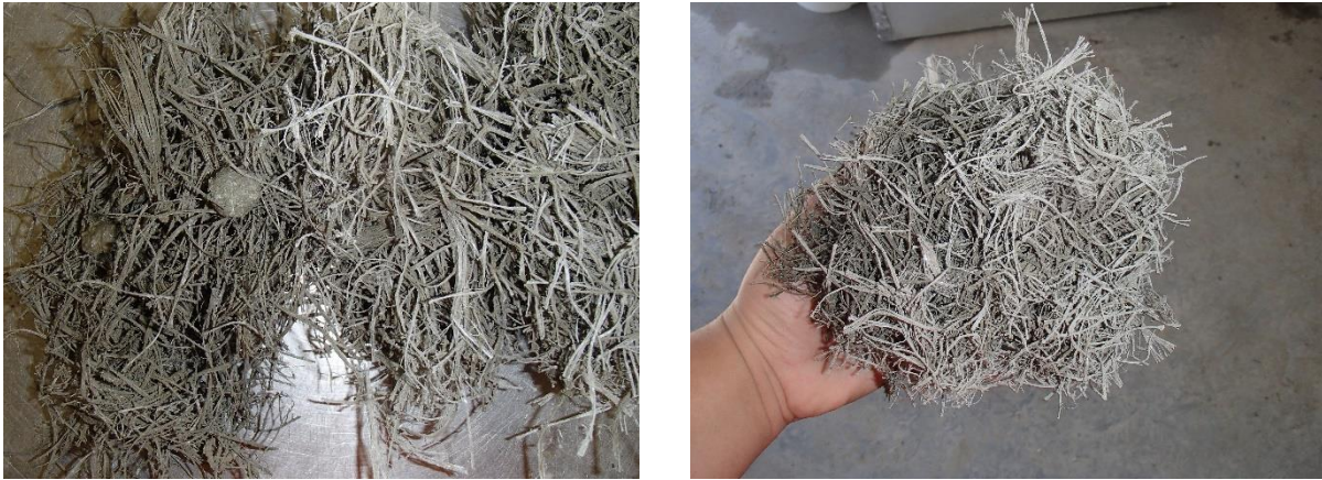
Figure G-5 Fiber clumping during mixing procedures (PP2-70)
