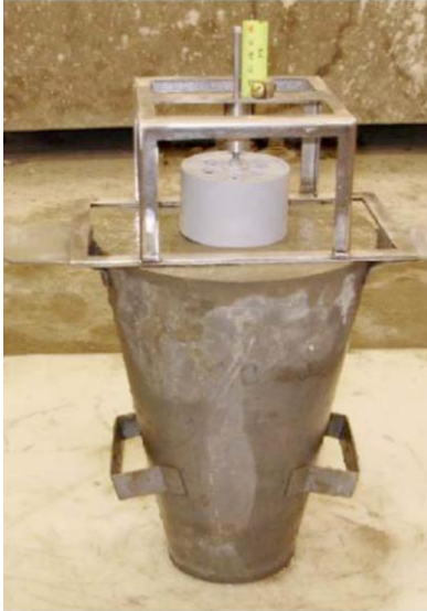
Figure A-5 Test setup and penetration apparatus (ASTM C1712-14)
