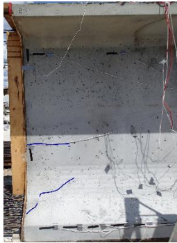
Figure 5-43 End region cracking after prestress transfer for PP-50 specimen: (a) analytical and (b) experimental.
