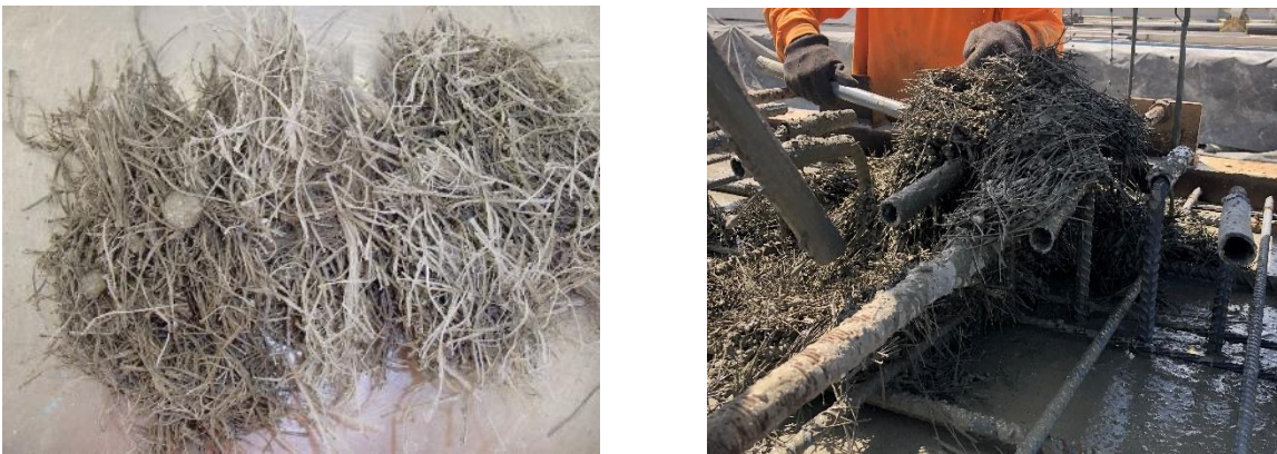
Figure 2-14 Fiber clumping during mixing (Macrosynthetic fiber with length 2.3 in. (58 mm) at volume of 0.7%)
