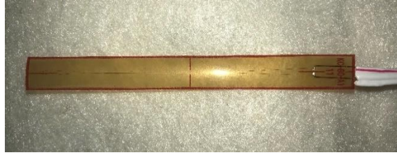
Figure 4-29 XS gages prior to installation
