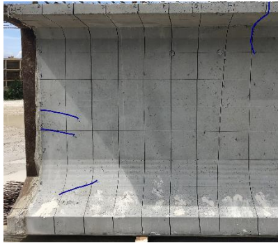
Figure 5-41 End region cracking after prestress transfer for SH-70 specimen: (a) analytical and (b) experimental.
