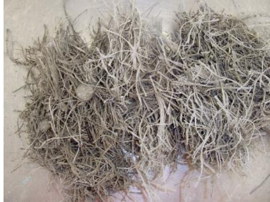
Figure 3-7 Fiber clumping during mixing procedures (Mixture 8)
