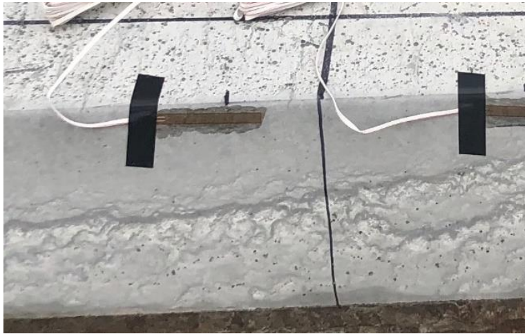
Figure 4-30 XS strain gages
