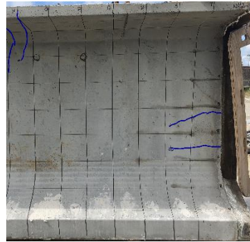
Figure 5-41 End region cracking after prestress transfer for SH-70 specimen: (a) analytical and (b) experimental.
