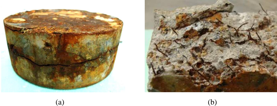
Figure 2-34 Micro crack in steel fiber-reinforced SCC samples (a) and fracture surface (b) (Frazão et al. 2015)
