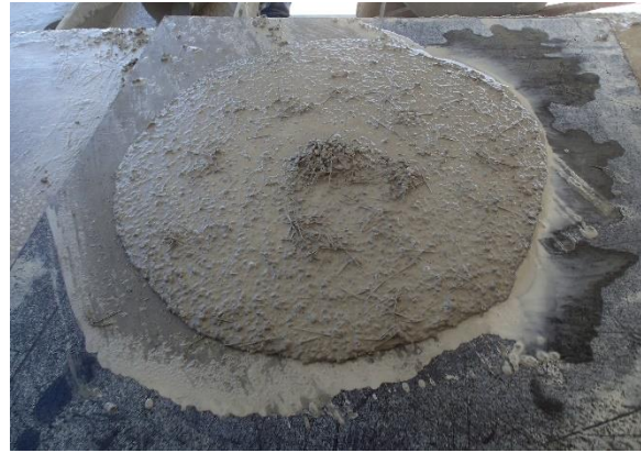
Figure G-3 Slump flow for (a) CR-70 and (b) PP-100
