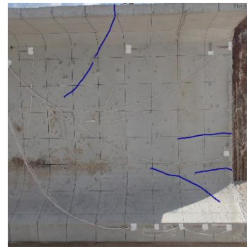
Figure 5-39 End region cracking after prestress transfer for CT specimen: (a) analytical and (b) experimental.
