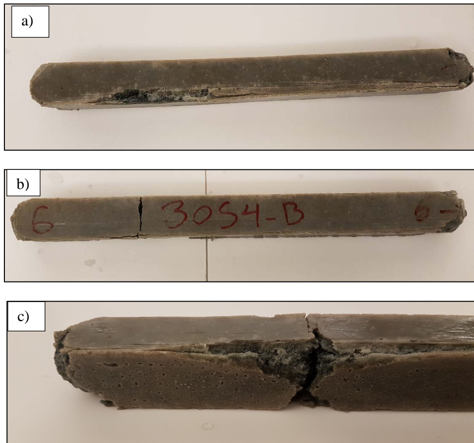
Figure 4-16: 30S16-B bars after a) 105 days and b) 120 days of exposure to 5% sodium sulfate solution; c) close-up view of the deterioration at 120 days.
