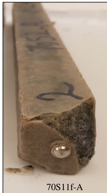
Figure 4-15: S11f-A bars at 1 year of exposure to 5% sodium sulfate solution
