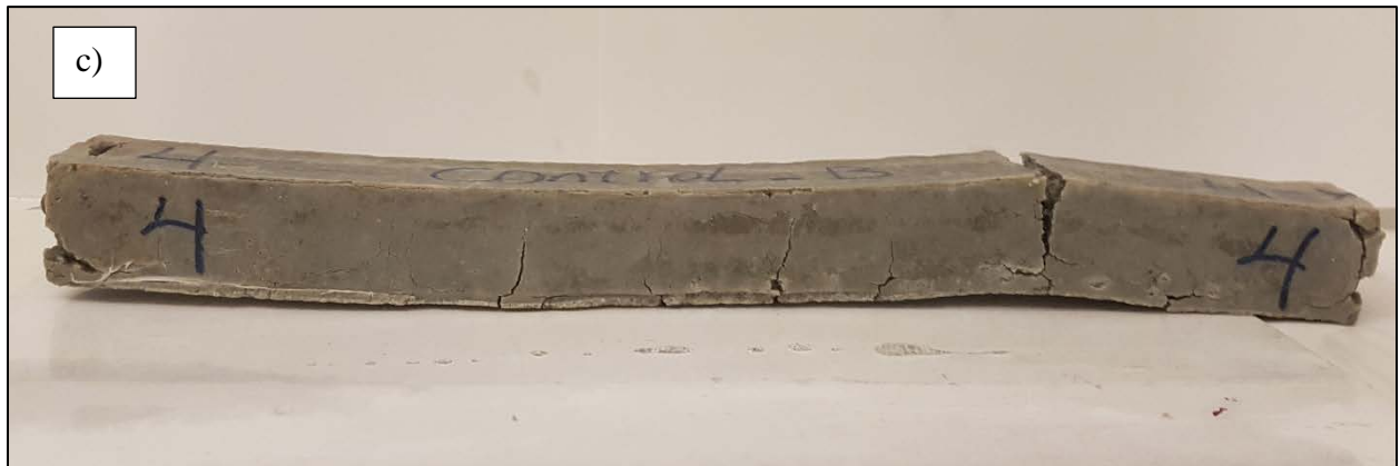
Figure 4-12: Control B sample after a) 91 days, b) 105 days and c) 120 days of exposure to 5% sodium sulfate solution
