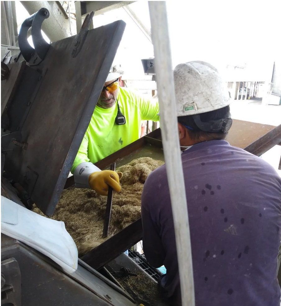
Figure 2-11: Workers avoid physical contact with fibers by using gloves and rods
