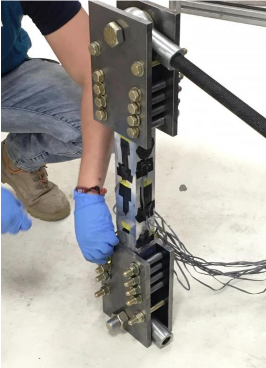
Figure 4-10: Aluminum Specimen in Tensile Grips
