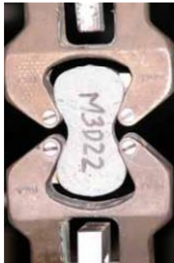
Figure 2-19: Mortar briquette specimen in tensile test machine. Image from (Graybeal 2006).
