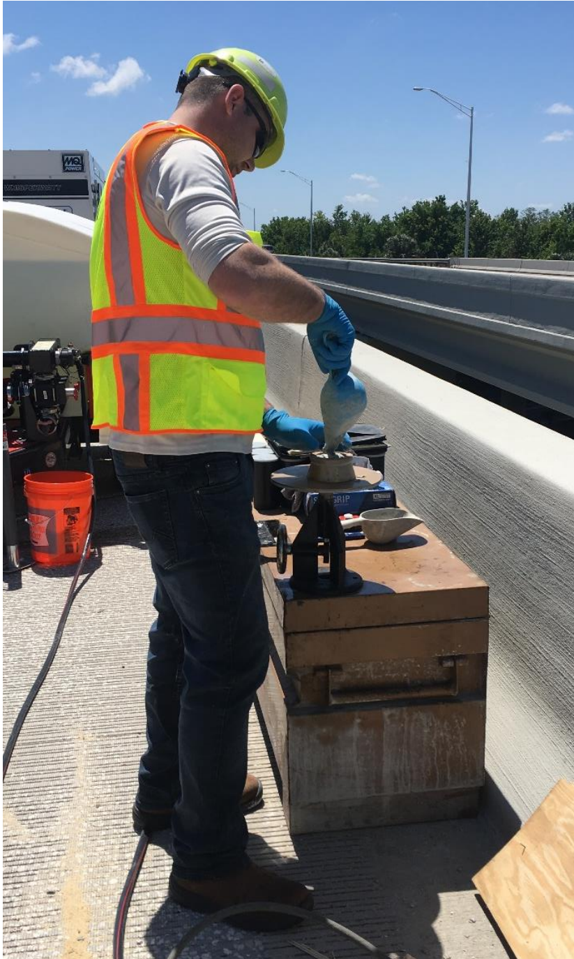
Figure 2-35: Mini slump test performed in field
