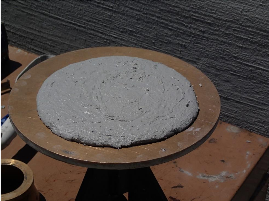
Figure 2-34: Final flow of UHPC
