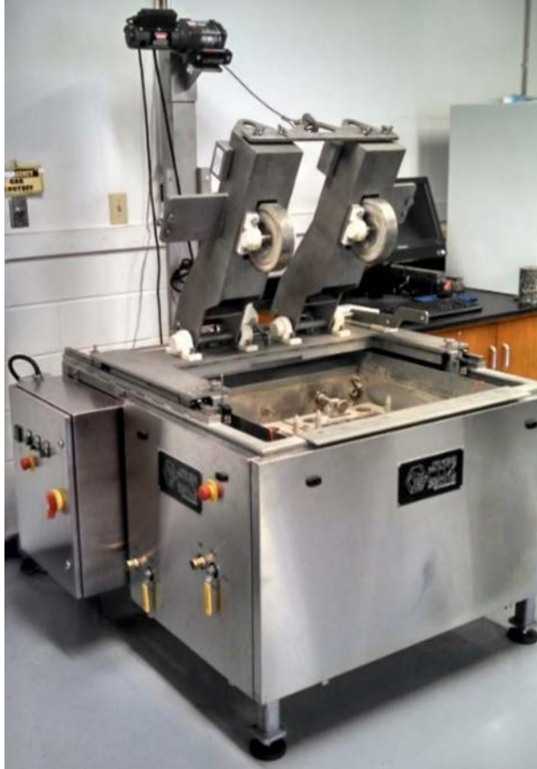
Figure 14. Hamburg Wheel Tracking Test Device
