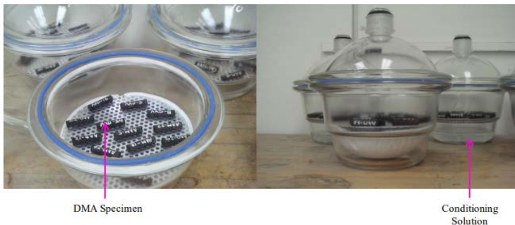
Figure 8. FAM Specimens Conditioned in Vacuum Desiccators (Tong, 2013)
