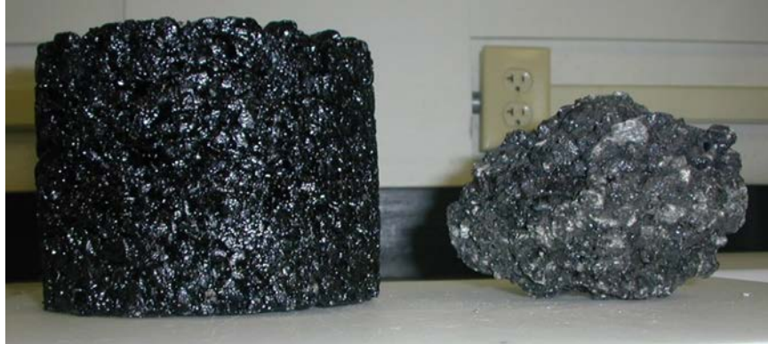
Figure 17. Cantabro Sample Before and After Testing
