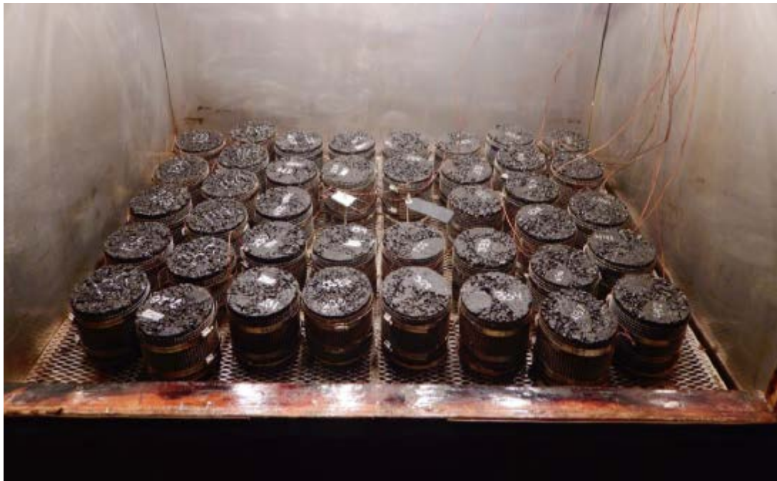
Figure 45. Photo of FC-5 Specimens in APWS Accelerated Aging
