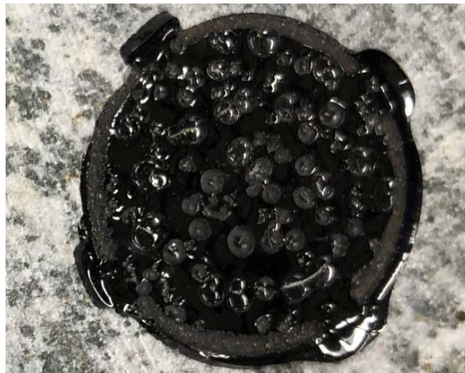
Figure 23. Cohesive Failure in the BBS Test
