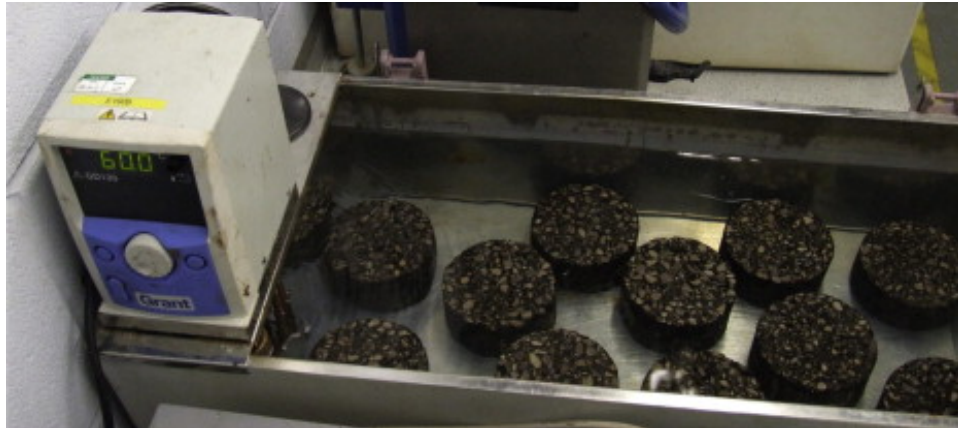
Figure 4. Asphalt Mixtures Conditioned in a Hot Water Bath (Apeageyi et al., 2014)
