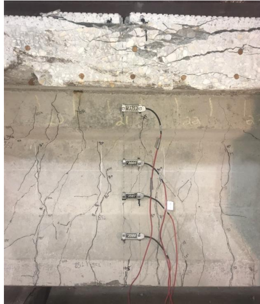
Figure 43. Crushing Failure in Top Slab of I-Beam 7
