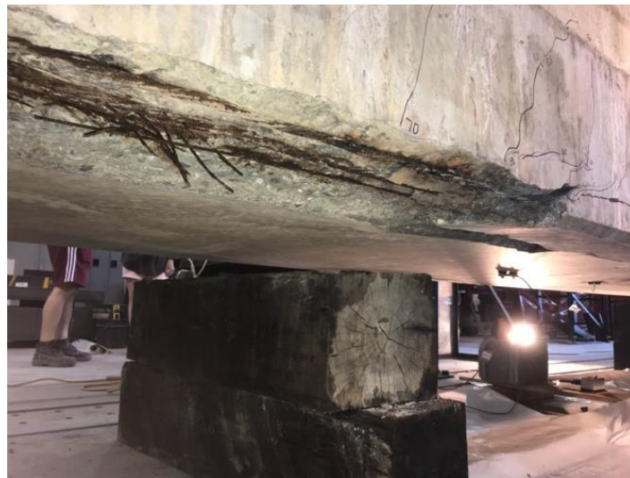
Figure 61. Condition of the West Side of Box Beam 1 Before the Test
