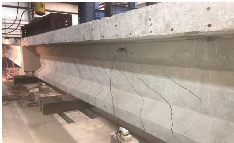
Figure 44. Residual Deflection after Testing I-Beam 7
