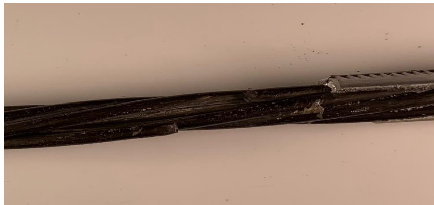
Figure 83. Strand Taken from I-Beam 7 after Testing
