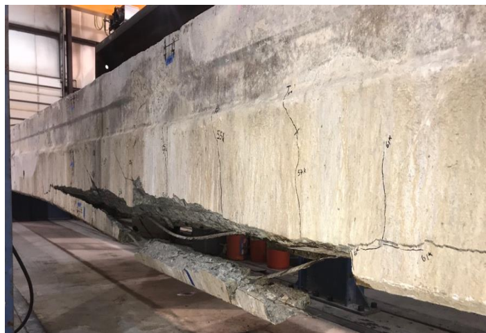
Figure 67. Box Beam 4 East Side after Testing
