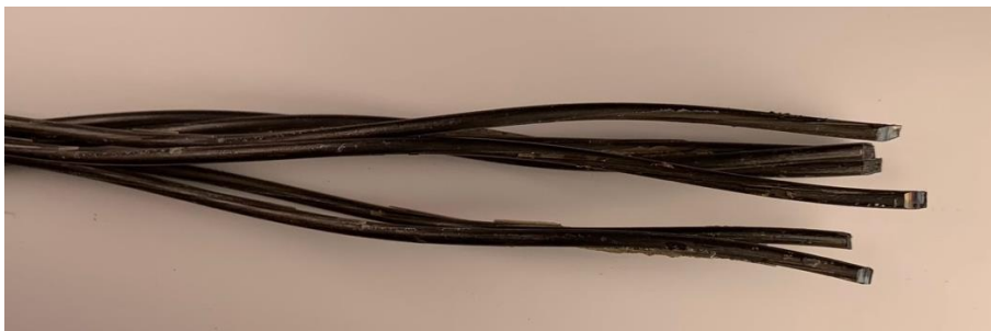
Figure 87. Strand Taken from I-Beam 3 after Testing
