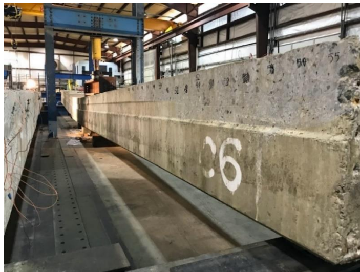
Figure 59. Large Deflection of Box Beam 1
