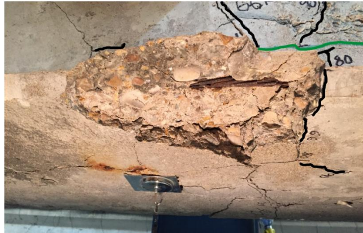
Figure 51. Hairline Crack Observed Prior to Testing (marked in green) Related to Corroded Strand Beneath on I-Beam 6
