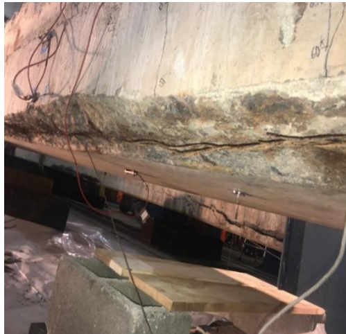
Figure 75. Corroded Strand on Bottom of Box Beam 2
