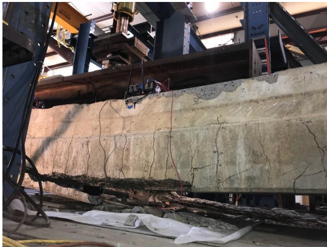
Figure 64. Condition of the East Side of Box Beam 1 at the End of the Test
