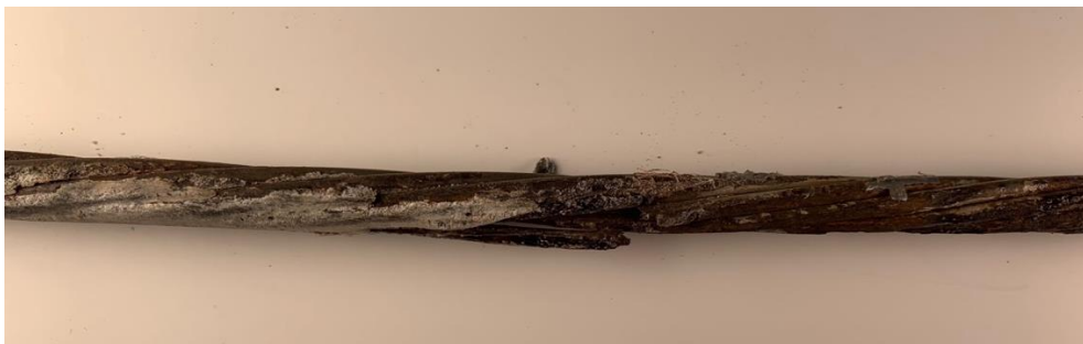
Figure 91. Strand Taken from Box Beam 4 after Testing
