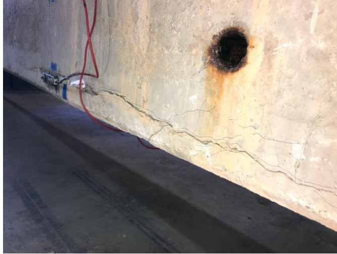
Figure 62. Condition of the East Side of Box Beam 1 Before the Test
