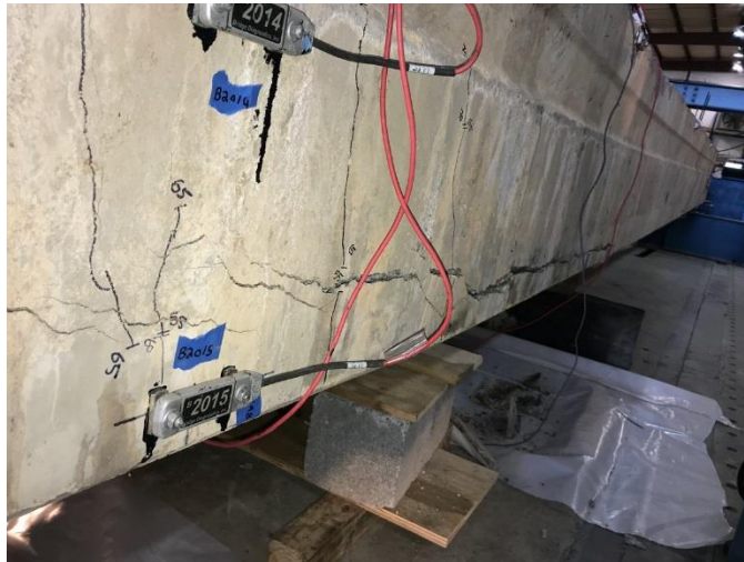
Figure 63. Propagation of the Cracks of the East Side of Box Beam 1 During the Test
