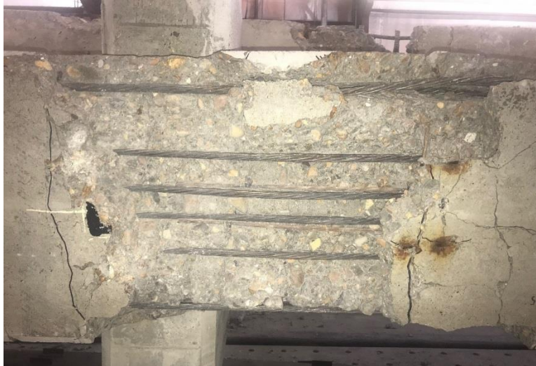
Figure 47. Bottom of I-Beam 7 after Testing
