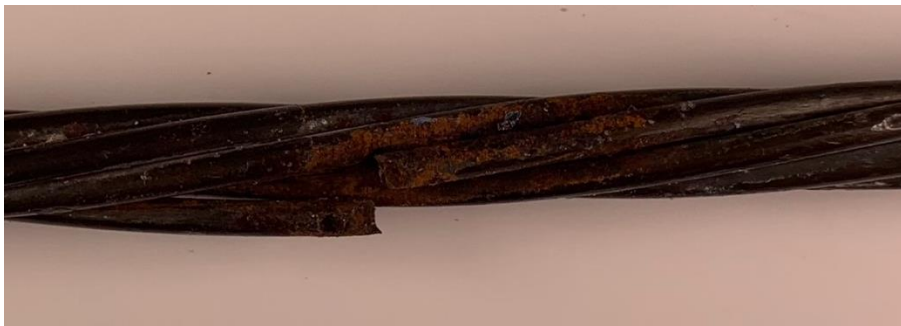
Figure 85. Strand Taken from I-Beam 6 after Testing
