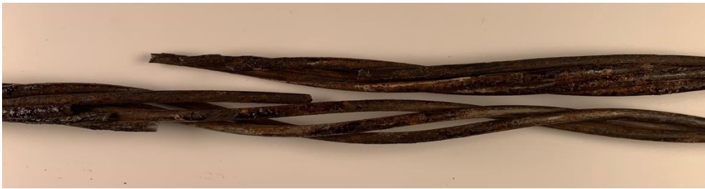
Figure 93. Strand Taken from Box Beam 2 after Testing
