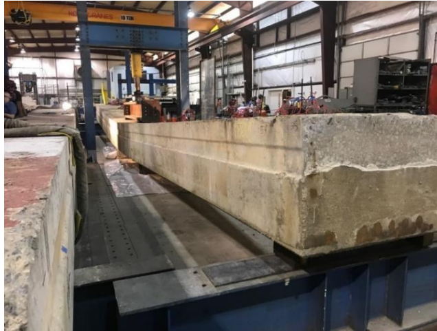
Figure 74. Large Displacement of Box Beam 2
