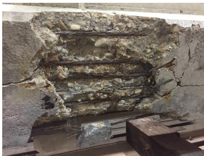
Figure 52. Bottom Flange of I-Beam 6 after Testing
