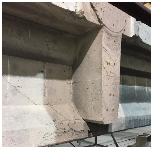
Figure 50. Cracking along Patch During Testing of I-Beam 6
