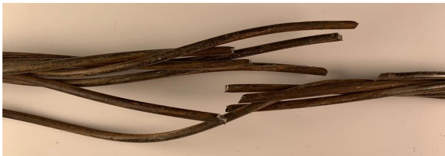
Figure 89. Strand Taken from Box Beam 1 after Testing
