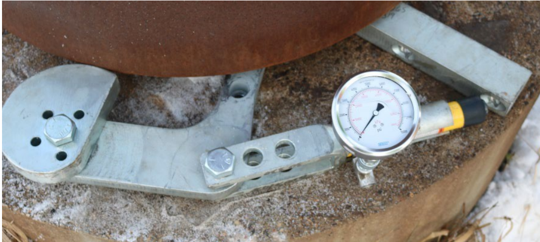
Figure 3.3.25 Millerbernd wrench operation at farthest setting
