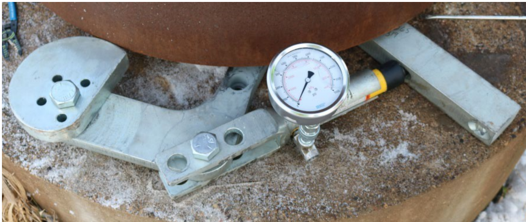
Figure 3.3.24 Millerbernd wrench operation at closest setting
