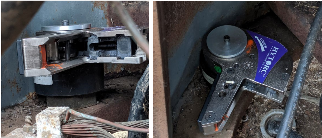
Figure 3.3.17 HYTORC Stealth 4 hydraulic wrench with stack socket
