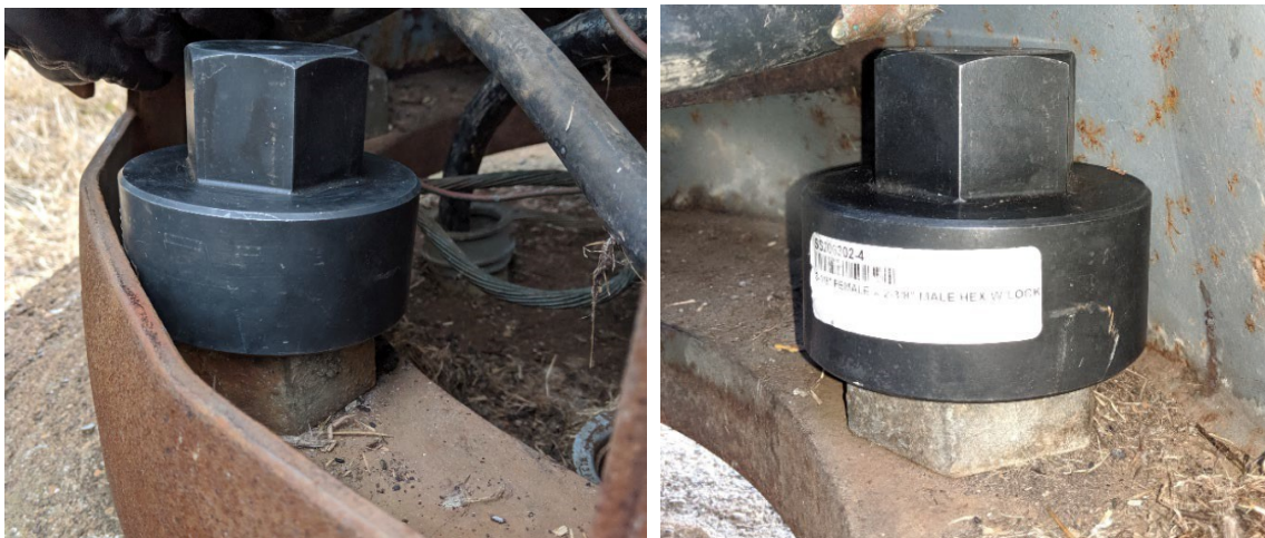
Figure 3.3.18 Wedging on door frame (left) and socket raised into wall by nut protrusion (right)
