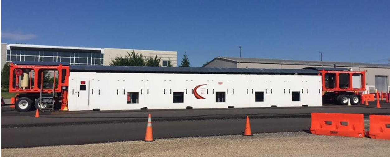
Figure A-2. Dynatest Mark VI Heavy Vehicle Simulator.
