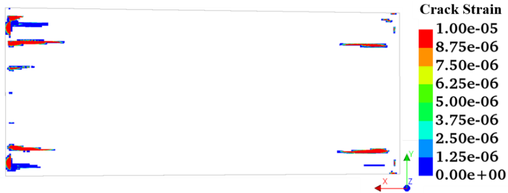
Figure 125 – Bottom view showing cracked elements in Inclined-FR.
