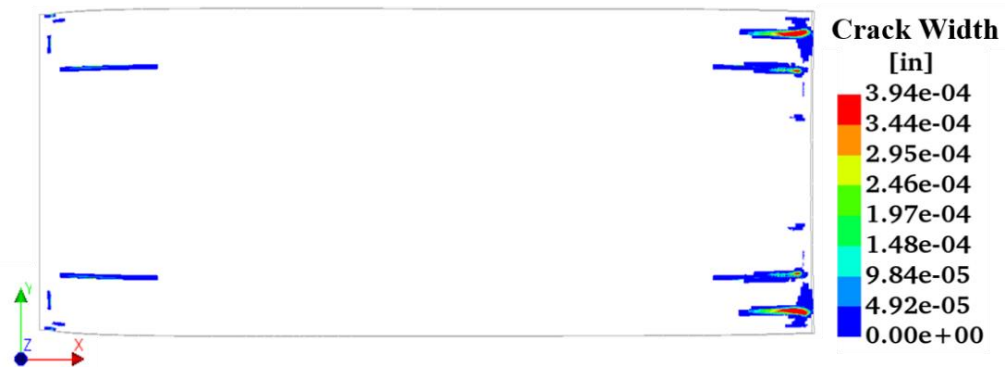
Figure 105 – Top view showing crack widths in Straight-FR.
