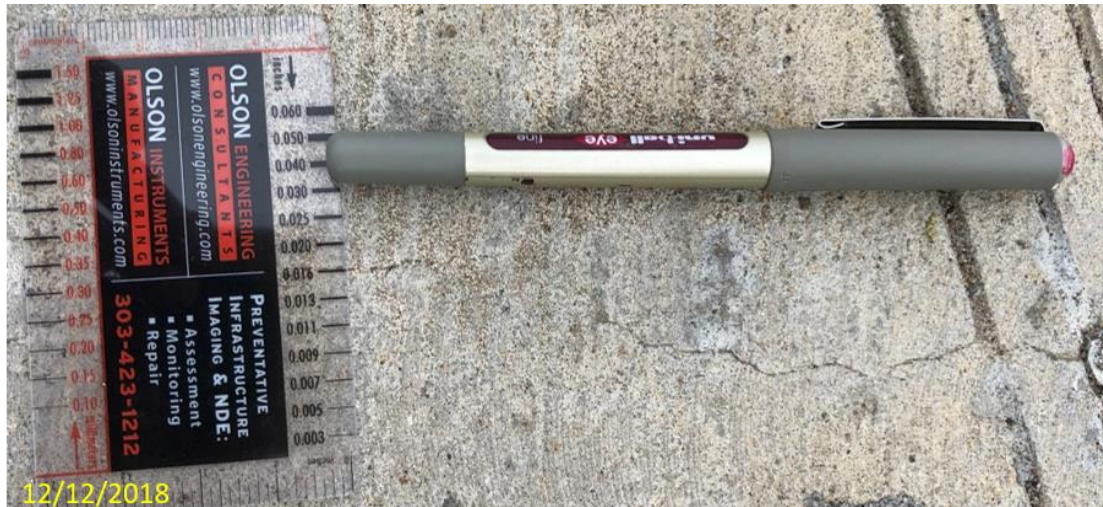
Figure 32 – Crack width measurement (0.016 in. or 0.41 mm).
