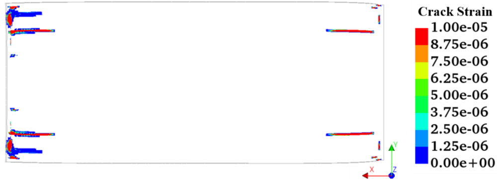
Figure 104 – Bottom view showing cracked elements in Straight-FR.
