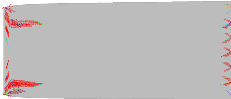
Figure 141 – Top view showing crack orientations in Inclined-VR.
