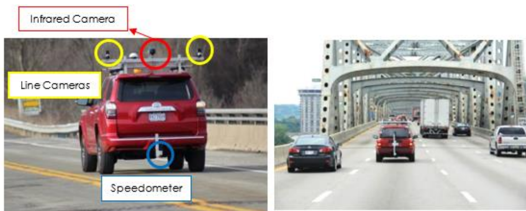
Figure 2a: The Deck Top Scanning System (DTSS)
