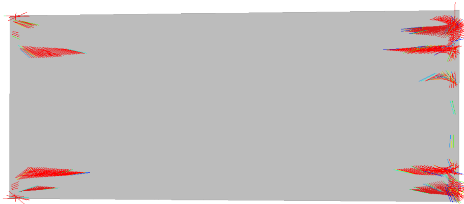
Figure 127 – Top view showing crack orientations in Inclined-FR.
