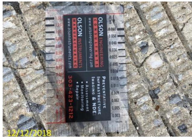
Figure 33 – Crack width measurement (0.020 in. or 0.51 mm).
