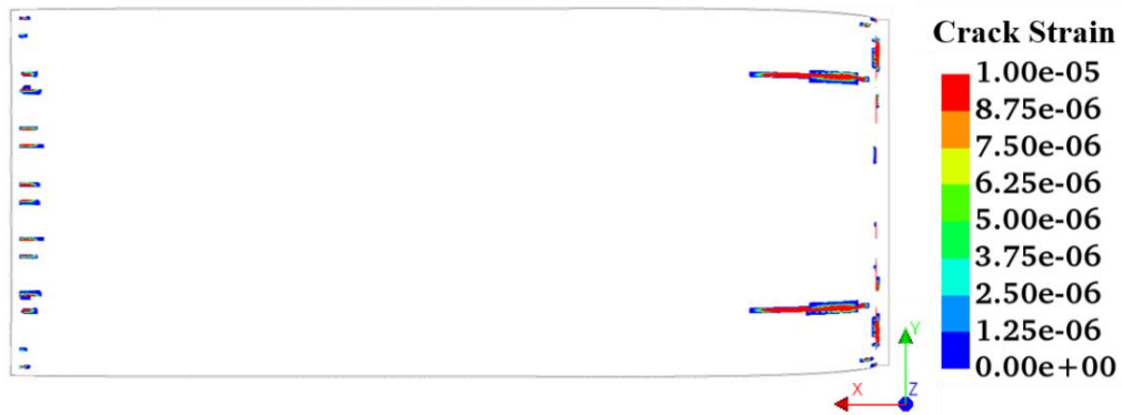
Figure 118 – Bottom view showing cracked elements in Straight-VR.
