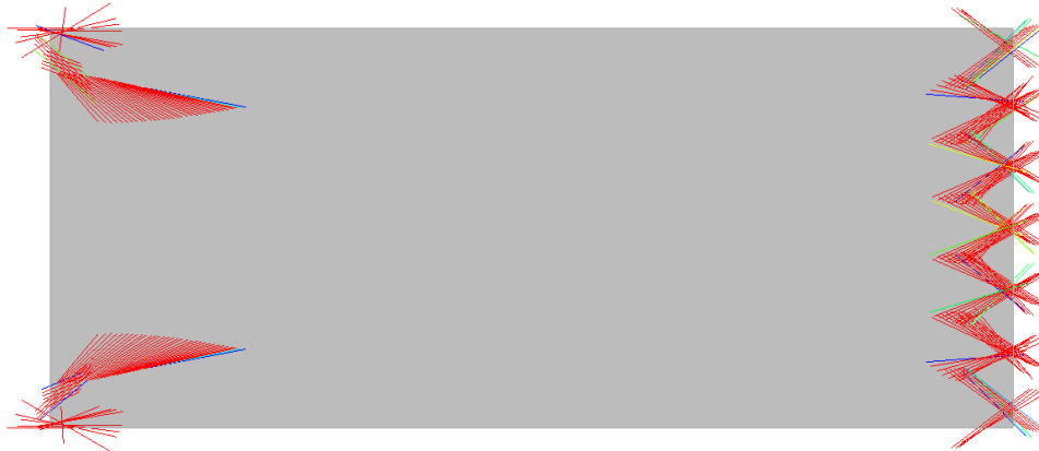
Figure 113 – Top view showing crack orientations in Straight-LVR.
