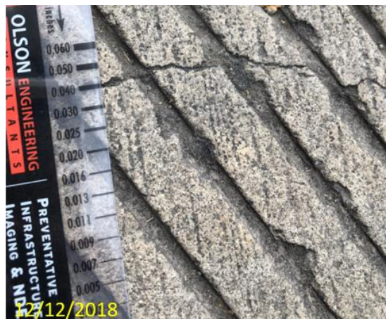
Figure 36 – Crack width measurement (0.040 in. or 1.02 mm).
