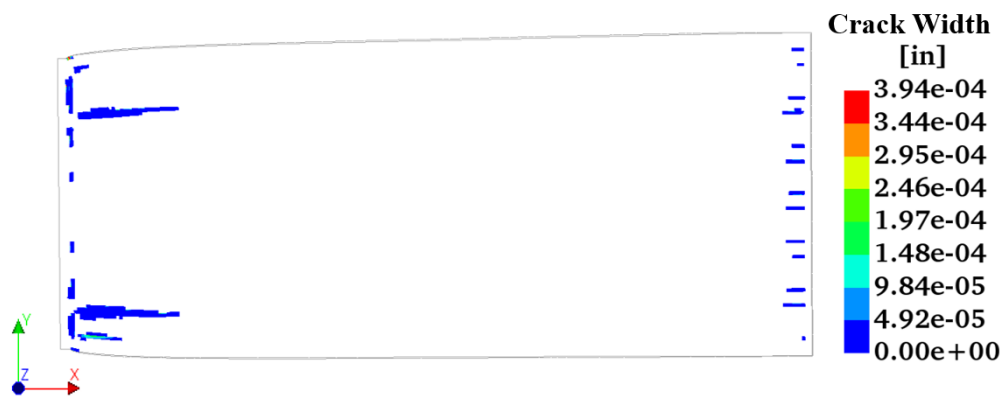
Figure 140 – Top view showing crack widths in Inclined-VR.
