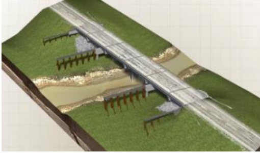
(a) Phase I of SPM construction: constructing substructure and placing temporary supports.
