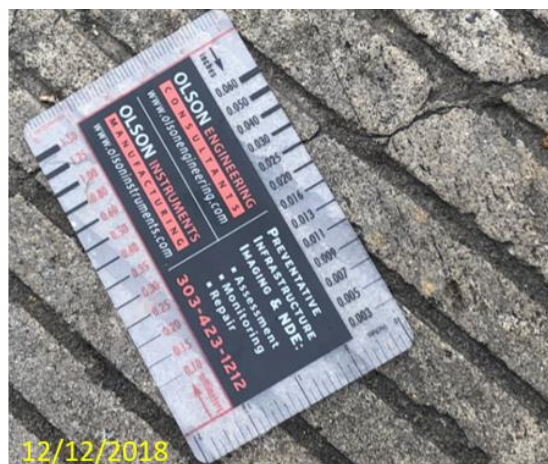
Figure 34 – Crack width measurement (0.025 in. or 0.64 mm).
