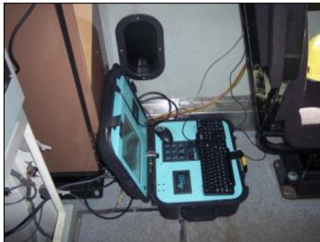
FIGURE 2-4. Installation of Axion PEMS inside the Locomotive Cab
