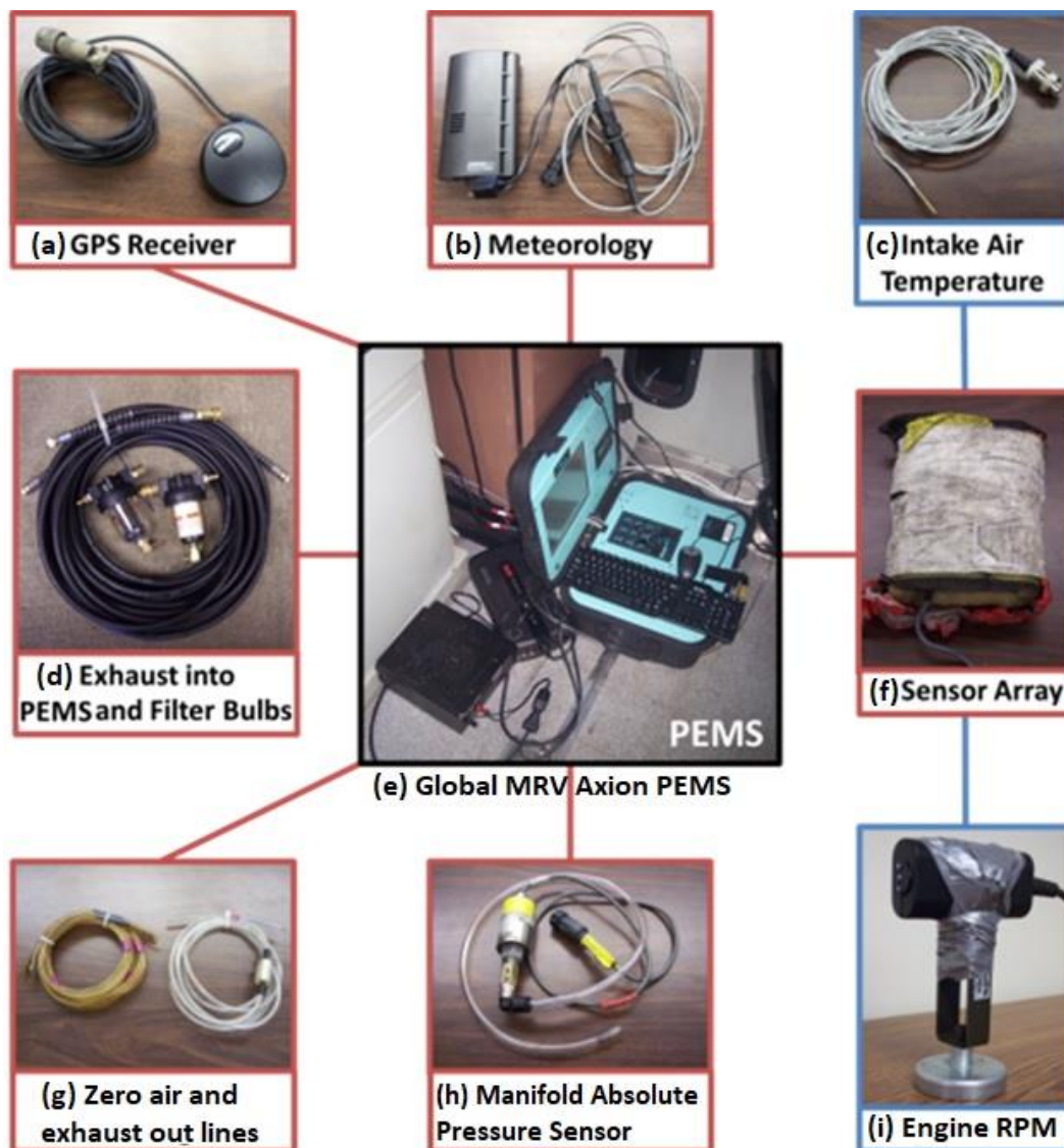
FIGURE 2-1. The Global MRV Axion PEMS and components: (a) GPS Receiver; (b) Meteorology Sensor; (c) Intake Air Temperature Sensor; (d) Exhaust Sample Lines; (e) Axion PEMS; (f) Engine Sensor Array; (g) Zero Air and Exhaust-out Lines; (h) Manifold Absolute Pressure Sensor; and (i) Engine RPM Sensor.
