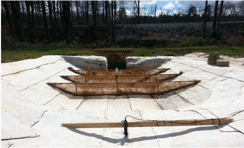
Figure C.1. Scaled sediment basin with baffles installed.
