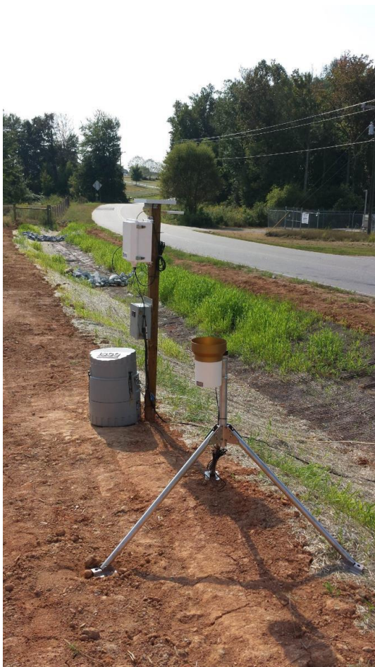
Figure B.8. Image of a “base station” installed at the upstate location, equipped with a rain gauge and cellular modem.
