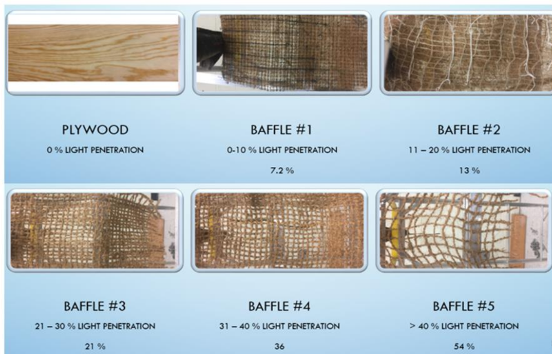
Figure 2.1. Various baffles tested with corresponding percent light penetration ratings.
