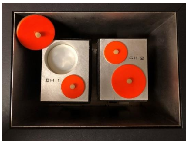
Figure 8 – Isothermal calorimeter used for HoH testing.
