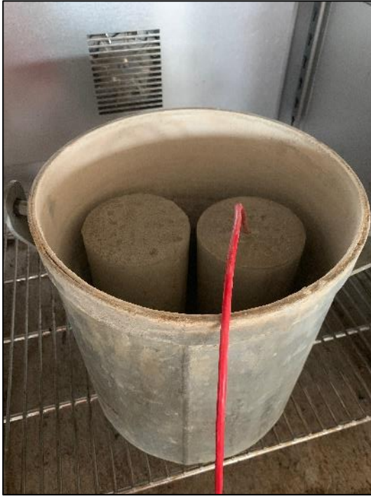
(a) cylinder with strain and temperature gauge
