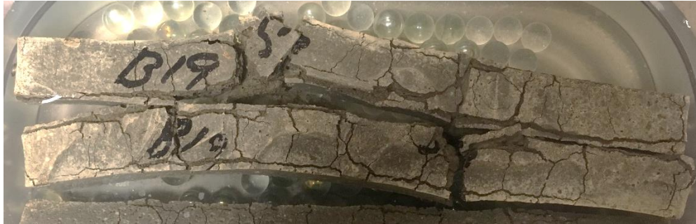
Figure 33 – Deleterious expansion by sulfate attack of MK2-10 mortar bars.
