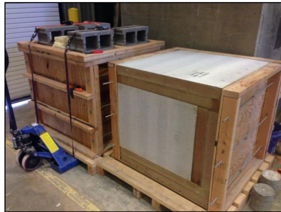
(e) adding top insulation and formwork and tightening the specimens
