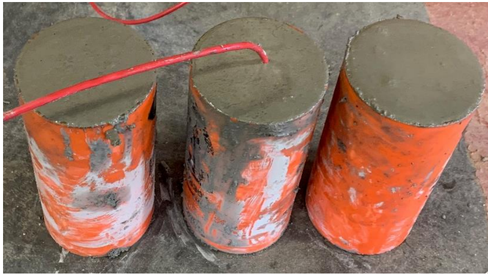
Figure E.1 – Casting concrete specimens with strain and temperature gauge.
