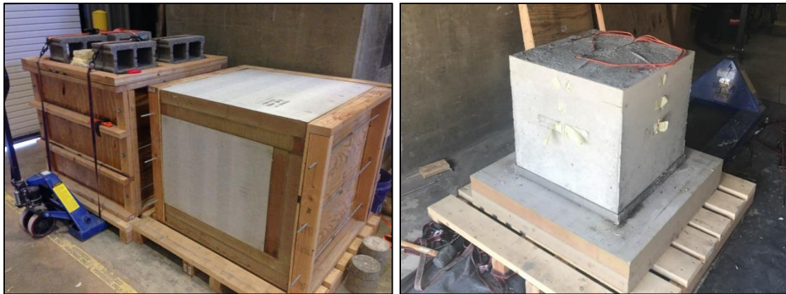
(a) formwork and insulation materials (b) cube specimen after formwork removal
