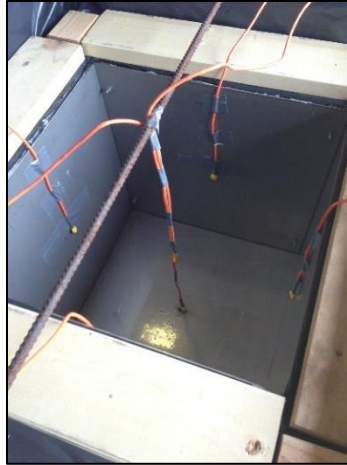
(b) thermocouples in the specimen
