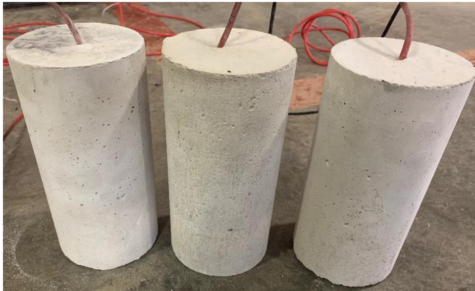
Figure E.3 – Concrete cylinders after being exposed to elevated temperature.
