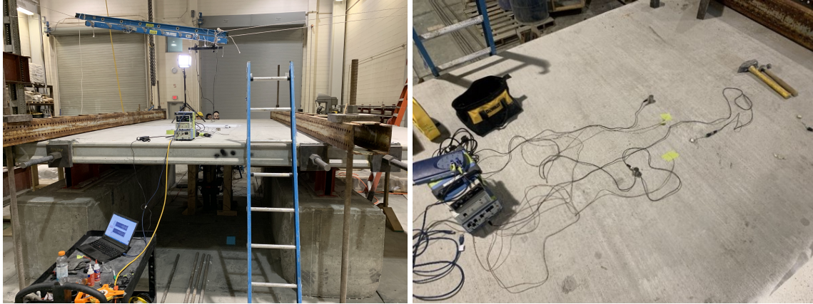
Fig. 4.7. Test on an one-way prestressed concrete slab in PKI structural laboratory to investigate the temperature effect on the ultrasonic wave velocity in prestressed concrete members.
