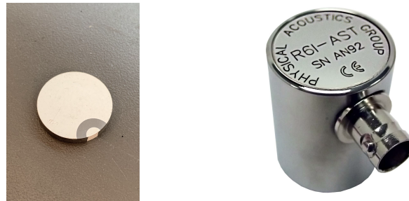
Fig. 3.2. Selected ultrasonic sensors: (a) PZT sensor from Steminc Inc. (b) AE sensor R61-AST from Physical Acoustic (Mistras).
