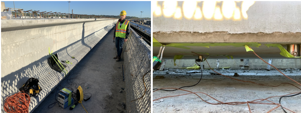
Fig. 4.6. Investigating temperature effect on ultrasonic wave velocity in the bridge girder.
