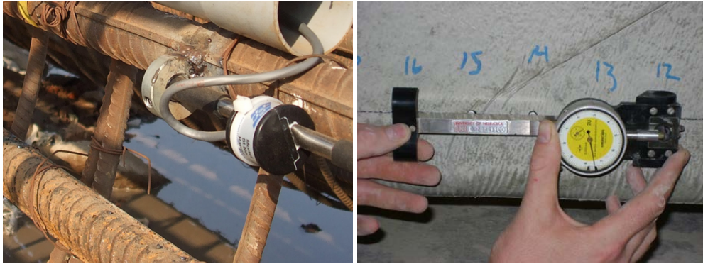
Fig. 1.1. Current methods for measuring prestress loss: a) embedded gauges, and b) surface gauges.
