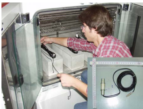
Fig. 2.2. Experimental setup of investigating the thermal effect on ultrasonic wave velocity change. Left figure presents the climate chamber with samples equipped with embedded ultrasonic sensors. Right figure shows the velocity variation due to temperature change in three samples [13].
