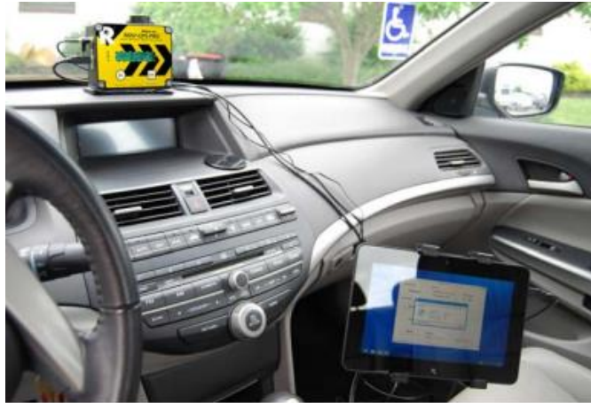
FIGURE 2-1. Photo. Rieker Inc.'s ball-bank indicator and the tablet device fitted into a data collection vehicle (Rieker Inc.)
