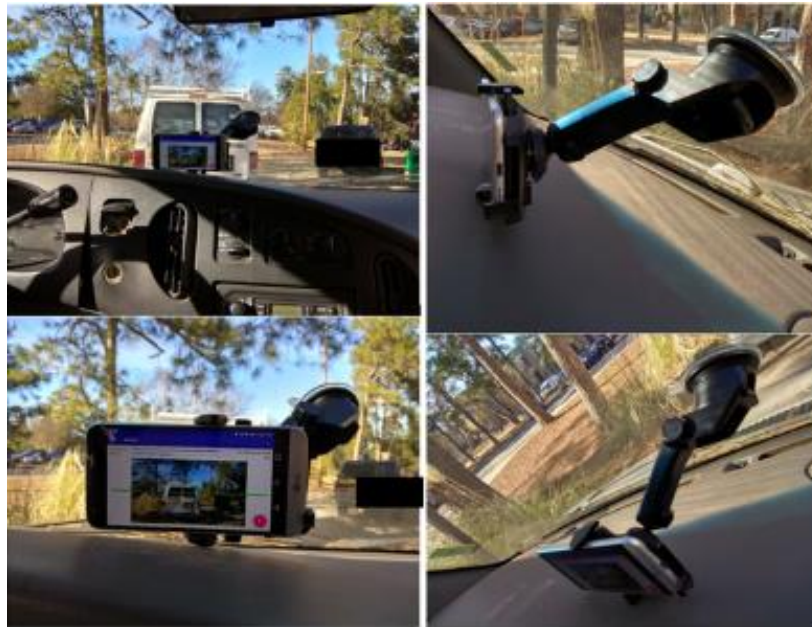
FIGURE 4-2. Photos. Different views of smartphone installation inside a vehicle
