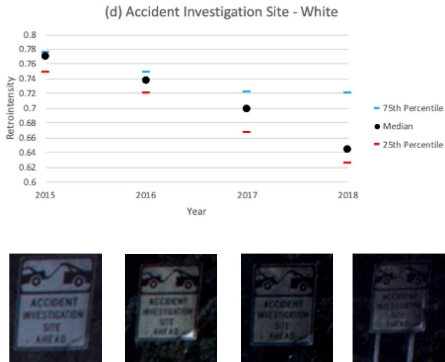
Figure 4-14. Multiple Elements. Retro-intensity over four years for white sign.
