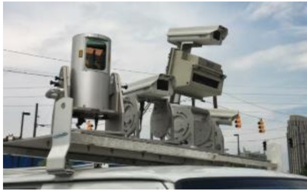
Figure 2-1. Photo. Mobile imaging sub-system on GTSV.
