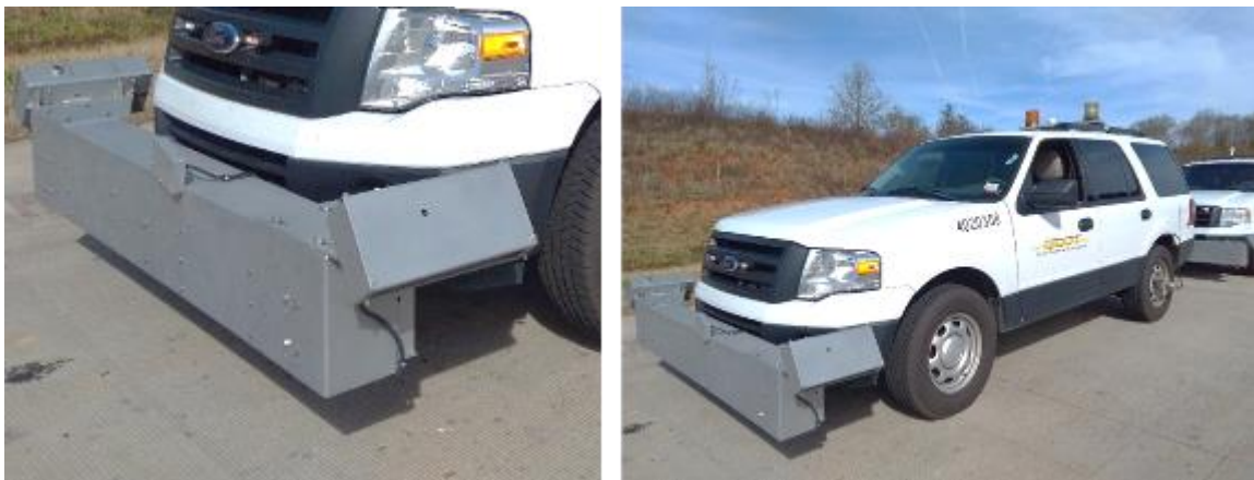
Figure 7-1. Photo. GDOT Profiler.
