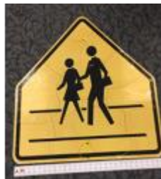
C. Subfigure of sign with cracked surface
