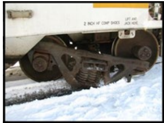
Figure 2. Broken side frame that led to derailment in winter
