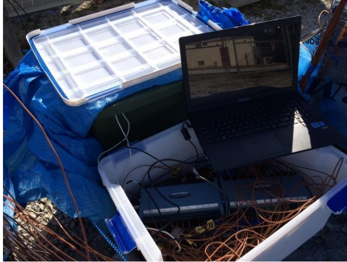
Figure 3.5 - Fayetteville Data Acquisition System – Measurement Computing USB-2416
