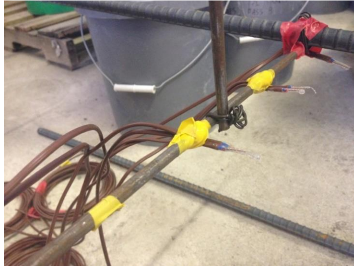
Figure 3.3 – Internal Type II thermocouples
