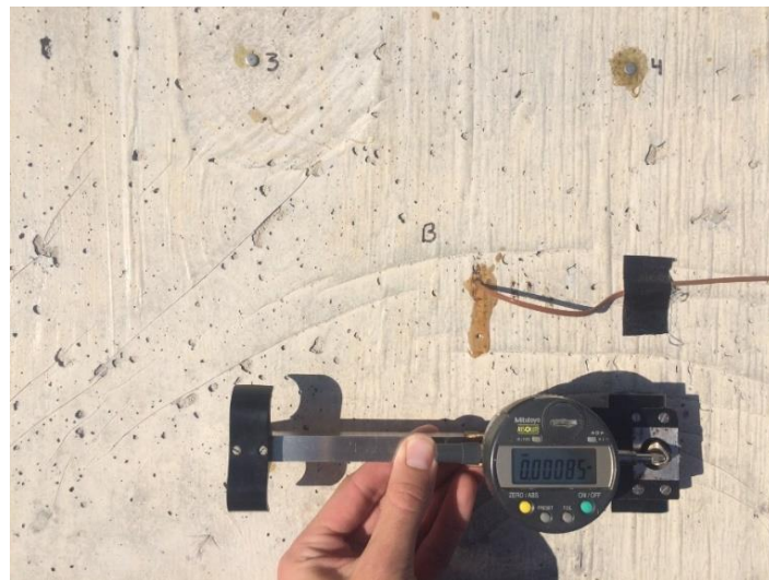
Figure 3.4 – Expansion/strain measurement with DEMEC gauge
