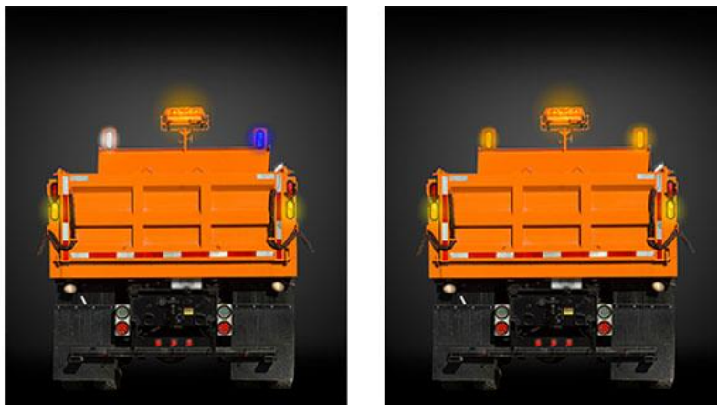
Figure 2-2 Color combination on snowplows to enhance safety: Left picture shows the latest blue lights on some snowplows and picture to the right shows enhanced amber lights on some DOT snowplows (Henderson, 2018).
