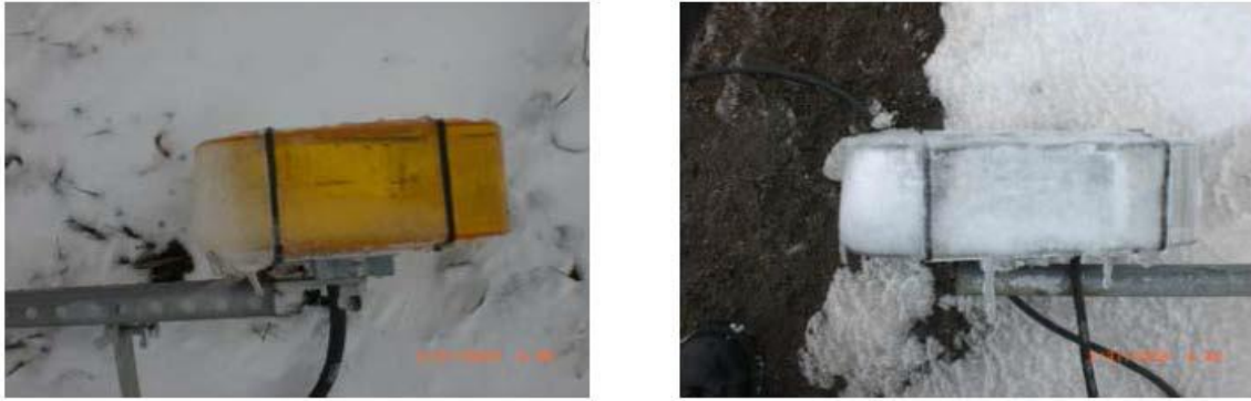
Figure 2-1 Comparison between HID (left) and LED (right) Lights after Heavy Snow Conditions (Vogt and Miller, 2008).
