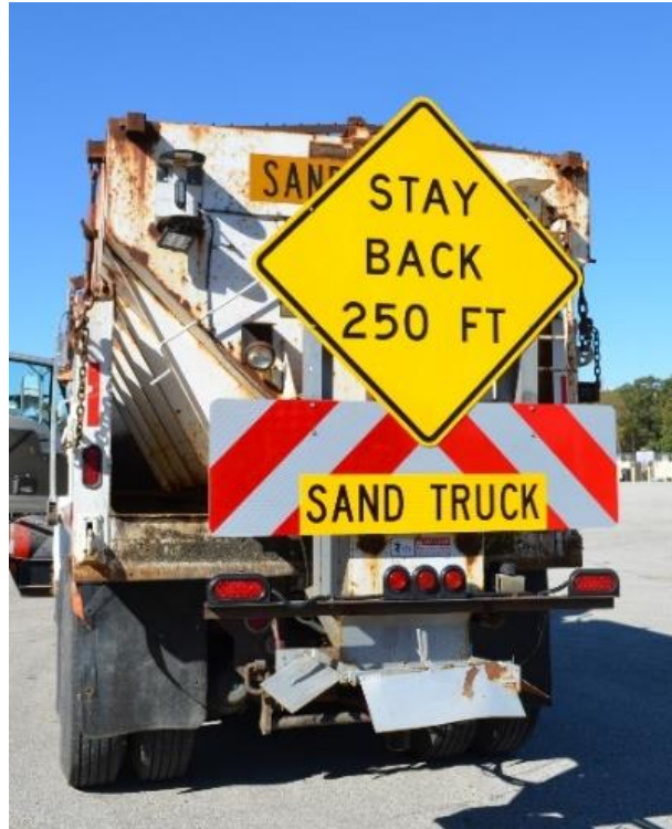
Figure 4-4 Message sign on back of winter operations vehicle in Paris District
