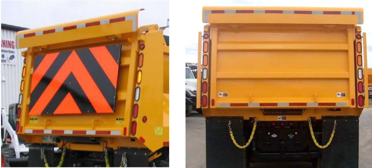
Figure 2-19 Red and white retroreflective tape fully outlining the rear tailgate of a winter operations vehicle in Ontario (Dow & Pearsall, 2014)
