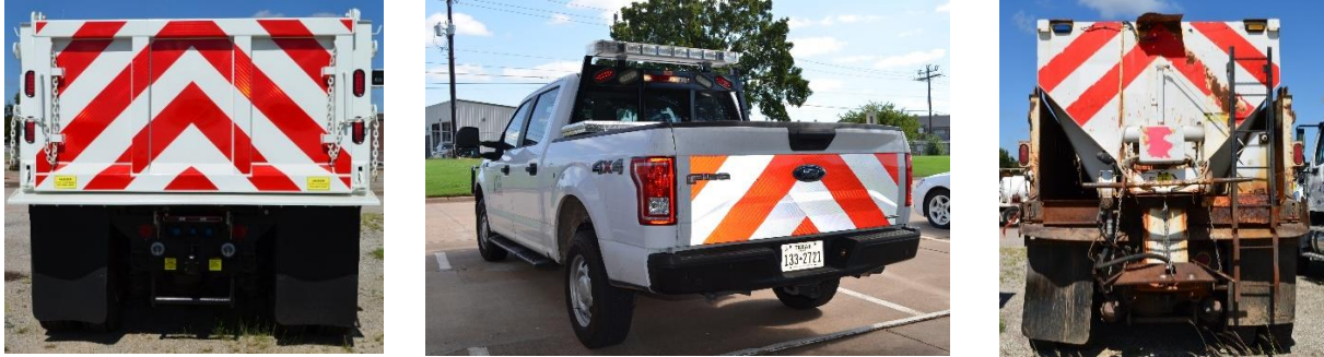
Figure 4-1 Chevron striped retroreflective markings on winter operations vehicle in Wichita Falls District
