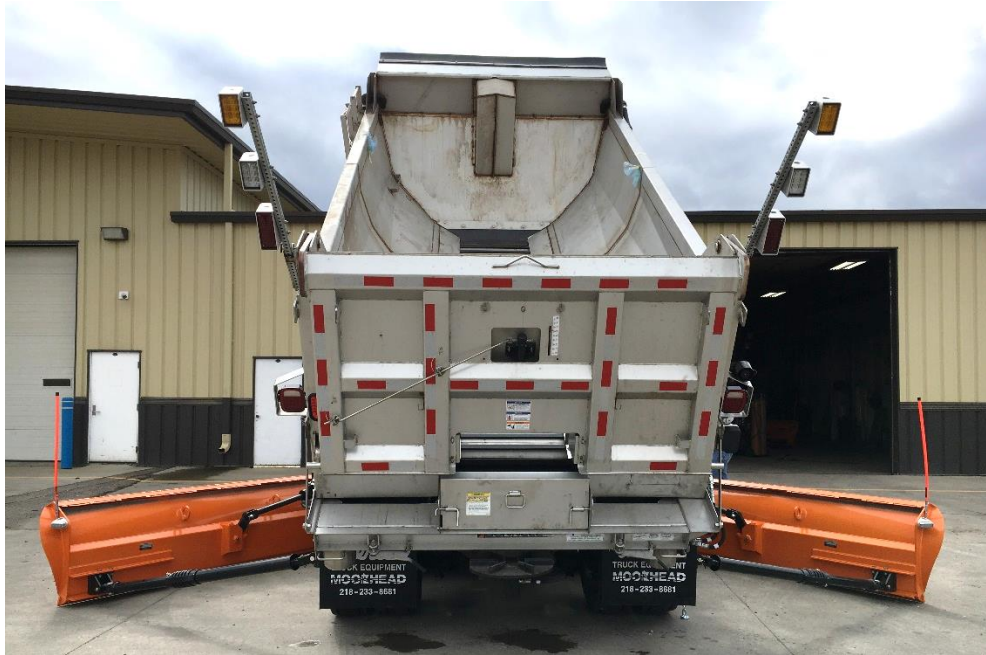
Figure 3-12 Back view showing wing plows of winter operations vehicles of North Dakota
