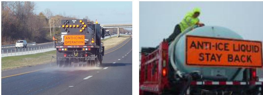
Figure 2-14 Anti-icing operations message signs on the back of winter operations vehicles in Kentucky and Kansas (Lake News, 2012 (left); KDOT, 2017 (right))
