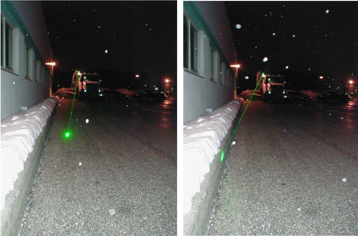
Figure 2-45 Laser projection in action showing outside edge of wing plow of a winter operations vehicle (Laserline, 2018)
