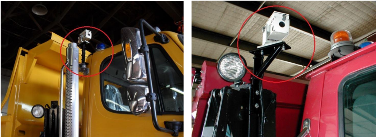
Figure 2-43 Two different winter operations vehicles with laser projection equipment installed on them (Laserline, 2018)
