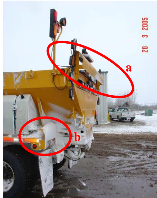
Figure 2-29 Side view of a winter operations vehicle showing: (a) Rear airfoil mounted on top of the vehicle and (b) Box wind deflector mounted on top of the taillight (Paulichuk, 2005)
