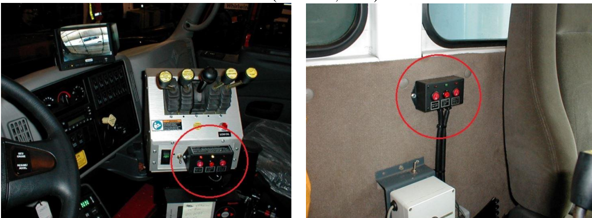
Figure 2-44 Laser control box inside of vehicles (Laserline, 2018)
