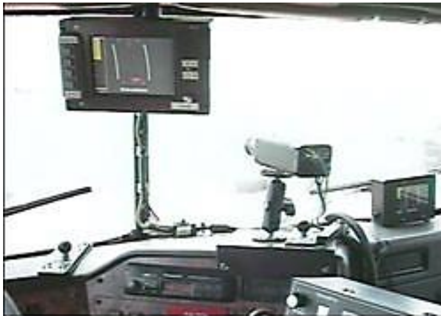
Figure 2-41 ASP Human-Machine Interface is mounted on the windshield of a Caltrans snowplow (FHWA, 2001)
