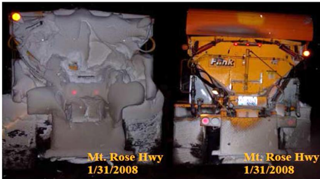
Figure 2-26 Airfoil test: Without airfoil and more snow accumulation on the rear (left) and with airfoil and less snow accumulation on the rear (right) (NDOT, 2008)
