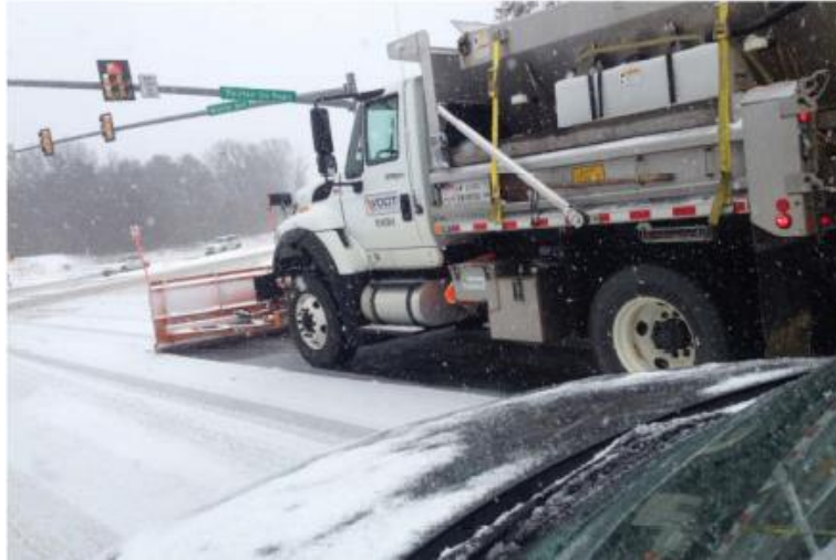
Figure 2-21 A winter operations vehicle of Virginia DOT with red and white retroreflective markings on the side (Washington Top News, 2015)
