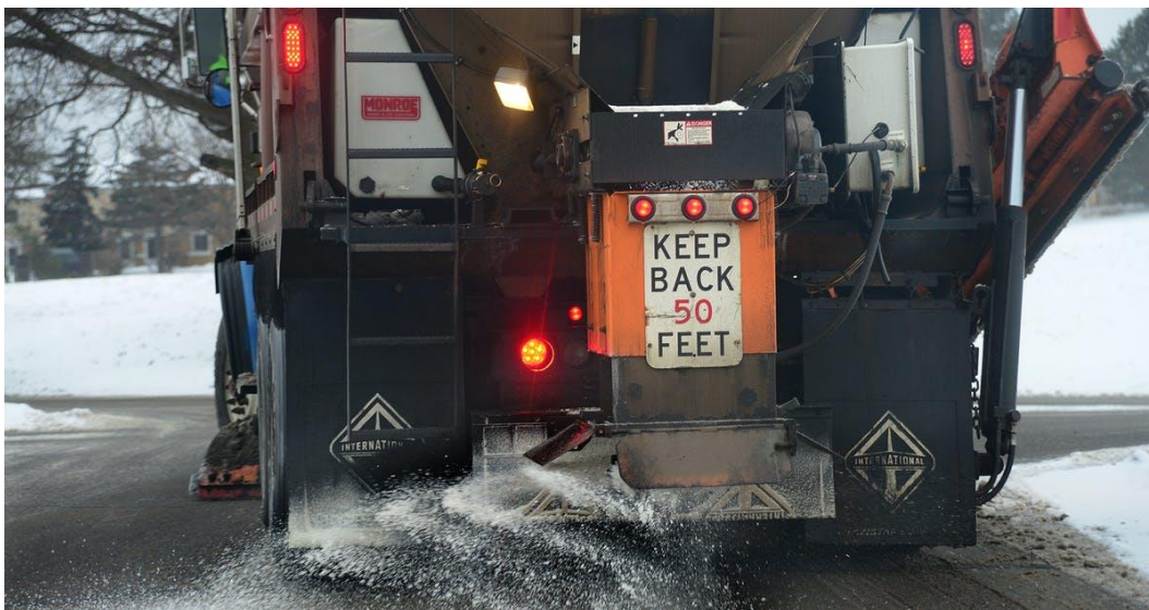
Figure 2-8 Message sign behind a winter operations vehicle in Minnesota (Star Tribune, 2017)
