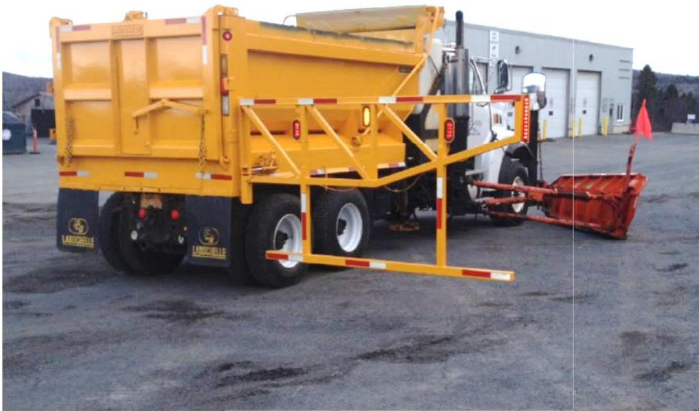
Figure 2-20 Safety Swing Arm with retroreflective markings (SNC Lavalin O&M, 2017)
