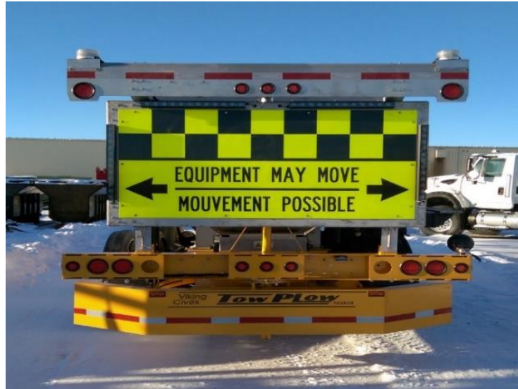
Figure 2-6 Message sign on the back of winter operations vehicles (MTO, 2015)
