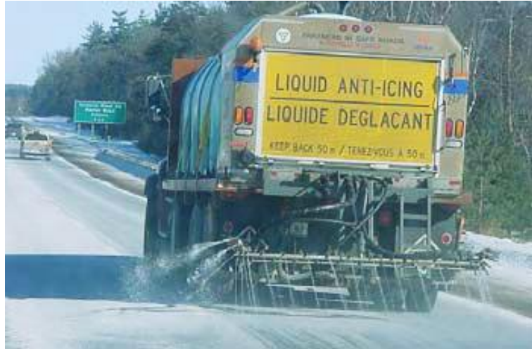
Figure 2-13 Anti-icing message sign on the back of a winter operations vehicle of MTO (MTO, 2018)
