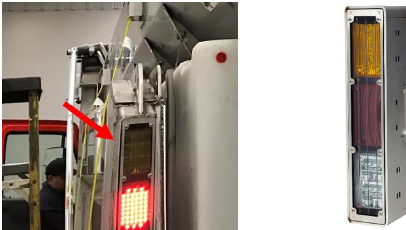
Figure 5-2 Recommended heated lens used with warning lights (Kansas)
