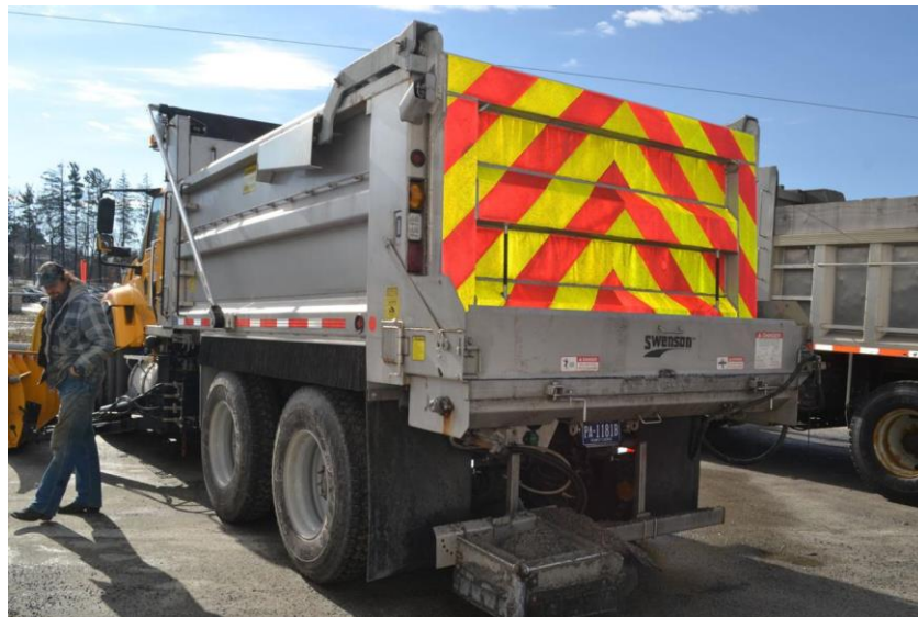
Figure 2-23 Warning sign on the back of a new winter operations vehicle in Pennsylvania (Daily American, 2017)
