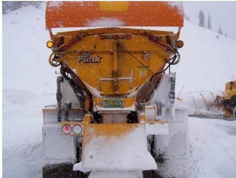
Figure 2-27 Airfoil keeping snow away from the back and left taillights of the winter operations vehicle but unable to keep snow away from right taillights. (NDOT, 2008)
