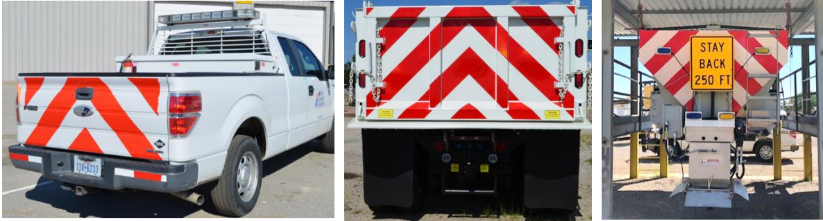
Figure 5-5 Recommended retroreflective markings on the back of winter operations vehicles (Paris (left), Wichita Falls (middle) and Dallas (right) Districts)
