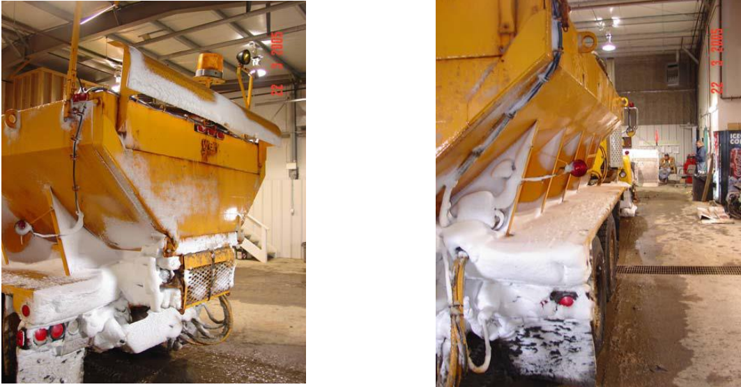
Figure 2-30 Wind deflector tests by Alberta Infrastructure and Transportation (Paulichuk, 2005) show extensive snow accumulation on the rear of a winter operations vehicle, despite having wind deflectors over taillights.
