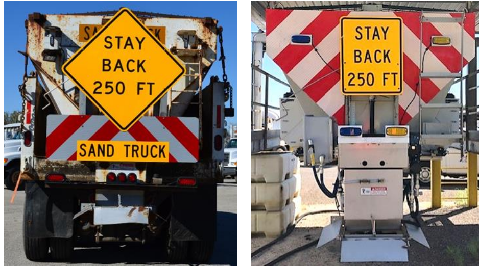
Figure 5-3 Recommended message signs on the back of winter operations vehicles (Paris District (left) and Dallas District (right))
