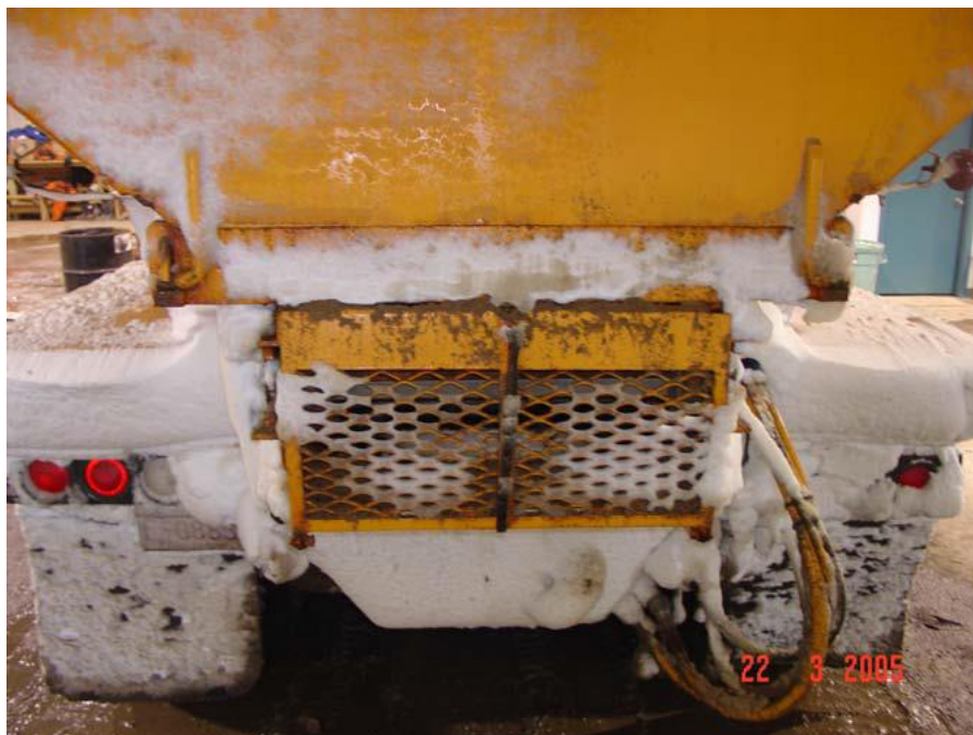
Figure 2-31 A direct comparison between the left and right taillights of a winter operations vehicle equipped with box wind deflectors. The right side is more heavily covered than the left side. (Paulichuk, 2005)
