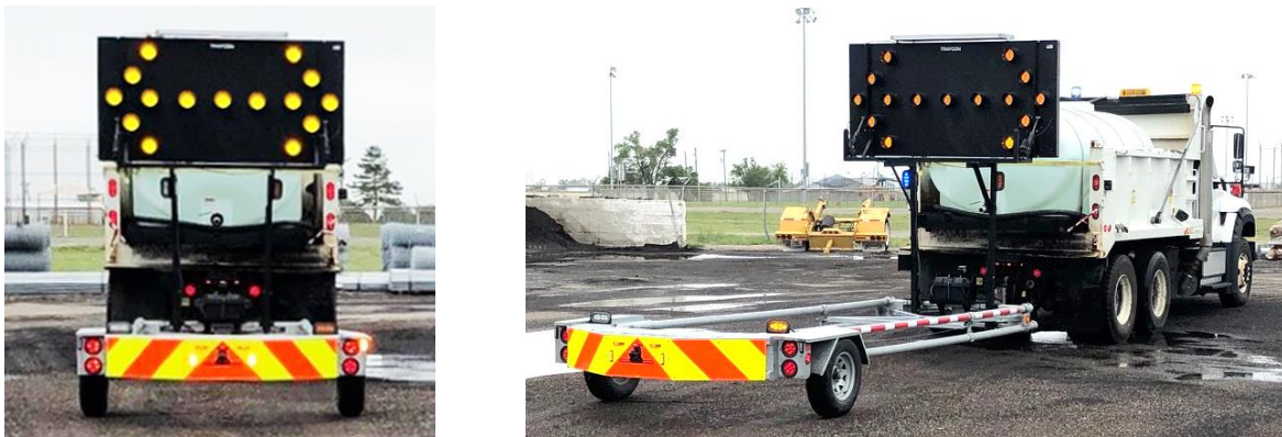
Figure 5-4 Recommended arrow board on the back of a winter operations vehicle (Amarillo District)
