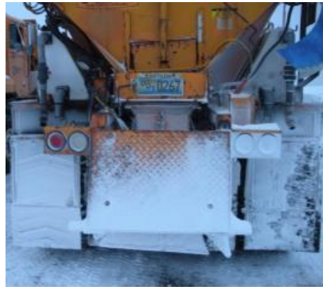
Figure 2-28 Side wind deflector on a winter operations vehicle (NDOT Class-15 Snowplow Truck) showing right taillight covered with snow despite the installation of the deflector (Dinc, 2011)
