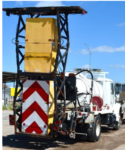
Figure 4-2 Truck mounted attenuator (TMA) mounted behind a winter operations vehicle in Wichita Falls District
