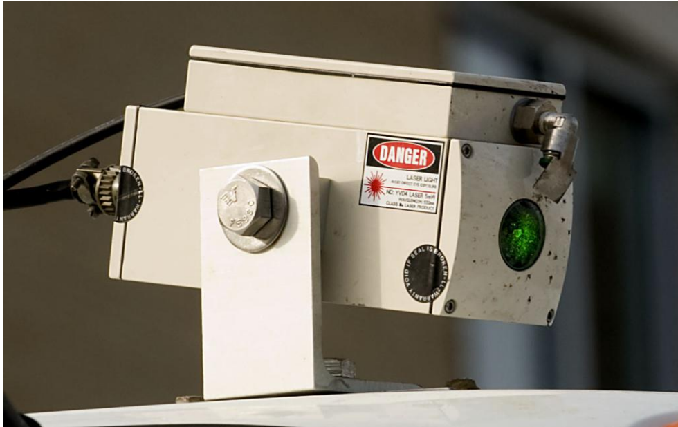
Figure 2-46 Bright green laser, as a guide to the trailing edges of snowplow trucks' wing plows, mounted on top of the trucks (Northern Virginia Daily, 2015)
