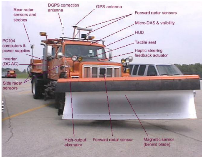
Figure 2-33 A winter operations vehicle of Minnesota DOT installed with equipment for HUD and GPS (Shankwitz & Preisen, 2015)
