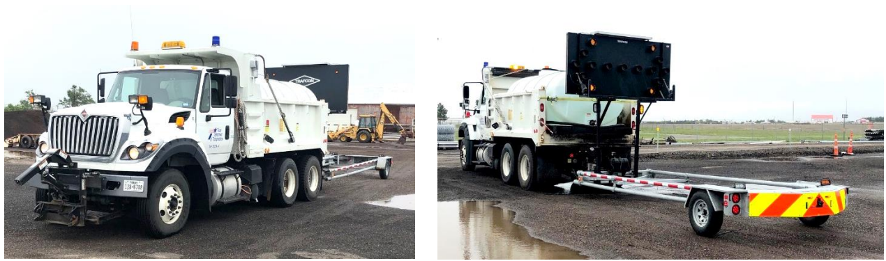
Figure 4-8 Front (left) and back (right) of winter operations vehicle attached to a TMA
