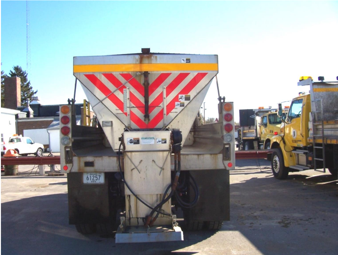
Figure 2-24 Warning sign on the back of Indiana DOT V-Box spreader (McCullouch and Stevens, 2008)
