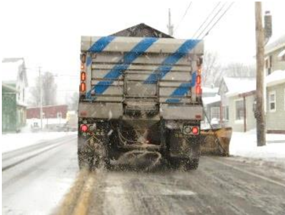
Figure 2-25 Warning signs on the back of a winter operations vehicle in Connecticut (CT Mirror, 2015)
