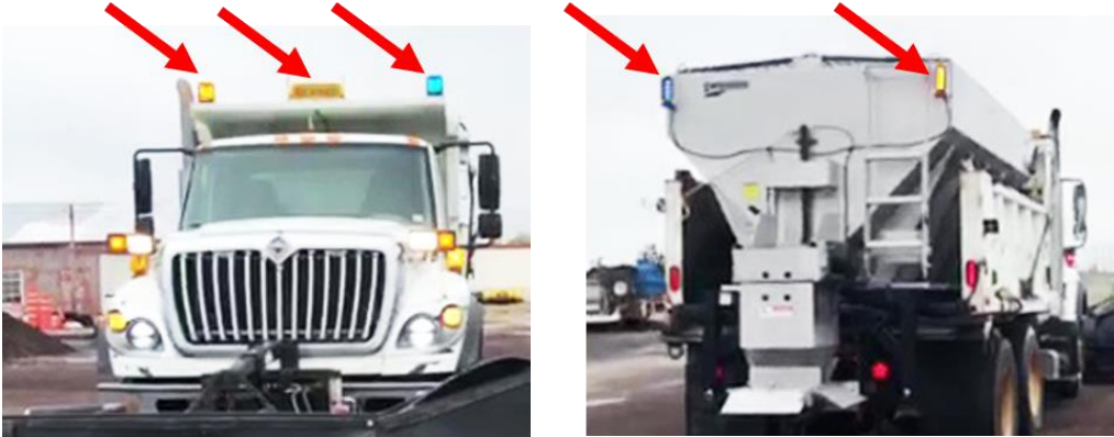
Figure 5-1 Recommended amber and blue color warning lights on top of winter operations vehicle (Amarillo District)
