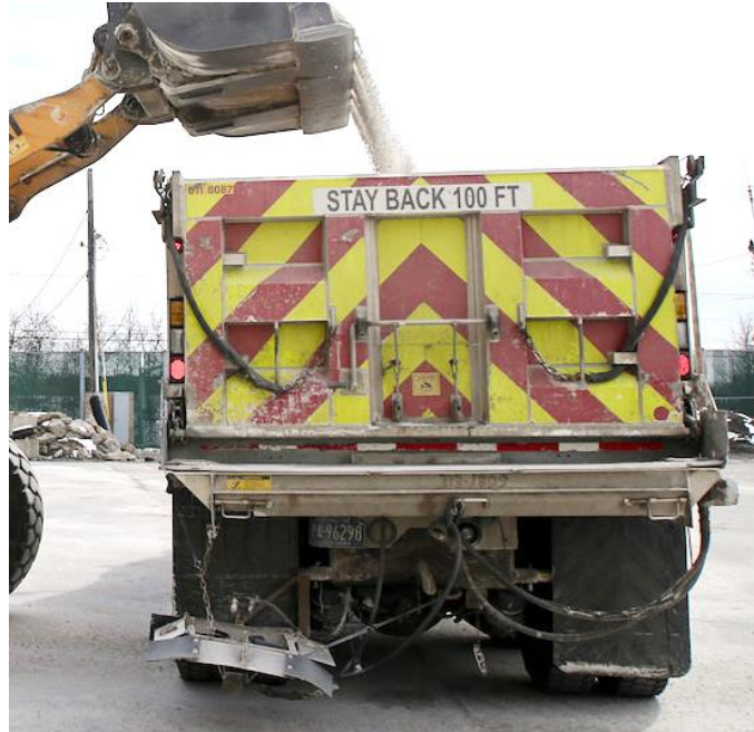
Figure 2-10 Message sign on the back of a winter operations vehicle in Pennsylvania (WITF, 2019)
