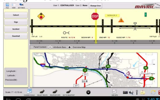
Figure 1. MAVRIC interface showing signs, culverts and guardrail features along the road network.
