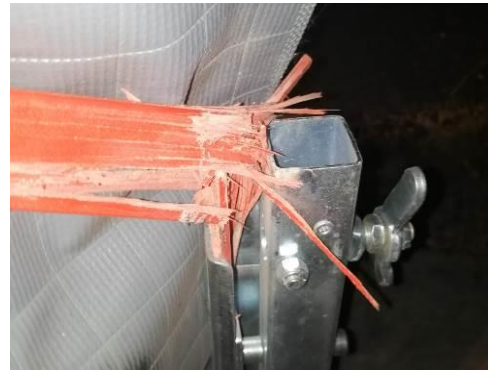
(b) Traffic Sign 1008 Main Body Broke
