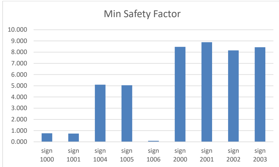
Figure 82. Minimum Safety Factor of Traffic Signs with 40 mph Wind Speed
