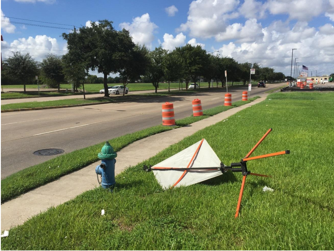
Figure 1. A Temporary sign knocked down by the wind on Bellaire Blvd, in Houston, Texas in 2018
