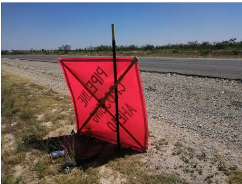
(a) Traffic Sign 2001 Fallen Down
