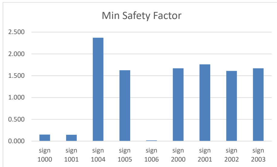
Figure 70. Minimum Safety Factor of Traffic Signs with 90 mph Wind Speed
