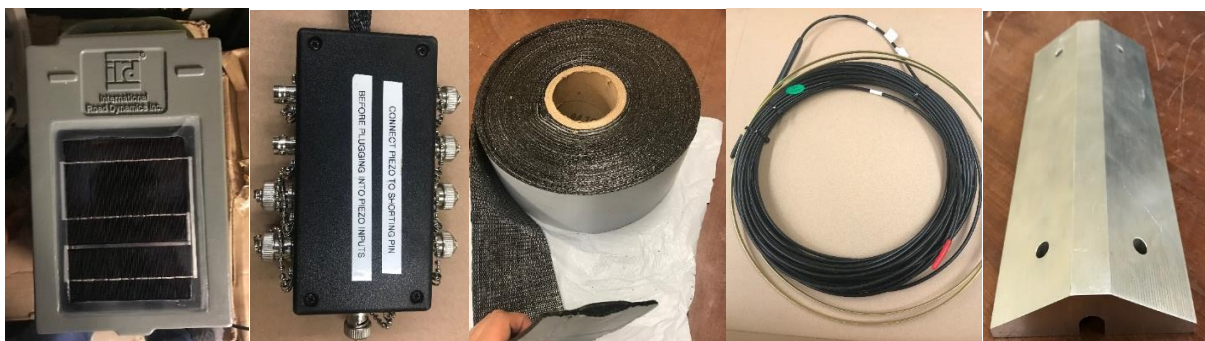
Figure 4.2. Field Equipment from Left to Right: TRS Controller, Piezo Input Box, 4in. Pocket Tape, Piezo-electric Sensors, Splice Protective Cover
