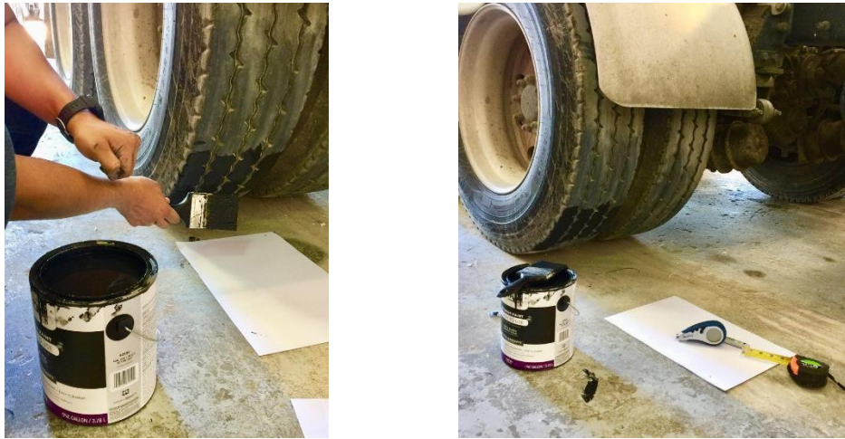
Figure 6.5. Painting Tires for Tire Footprint Measurement.
