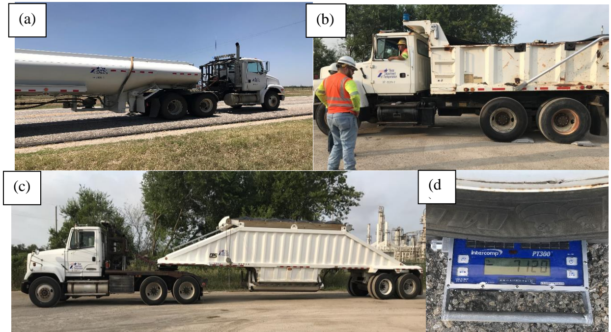
Figure 4.6. Static Axle Weight Measurements: (a) Class 6 Dump Truck (b) Class 9 Water Truck (c) Class 9 Belly Dump (d) Static Axle Weight Using Portable Scales.
